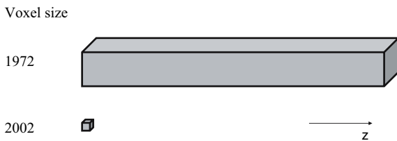
Fig. 2.2. Change in the size of a voxel element over the past 30 years
