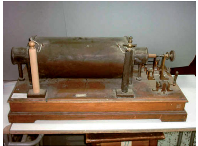
Figure 1.3 Inductorium device. Reprinted with permission from the Science and Technology Museum, University Junior College, Physics Department, Malta.
