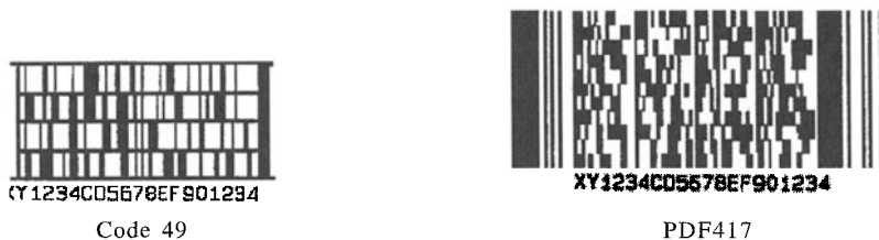
FIGURE 9-2. Representative stacked codes. Each layer is recognizable as a line of bar code.
