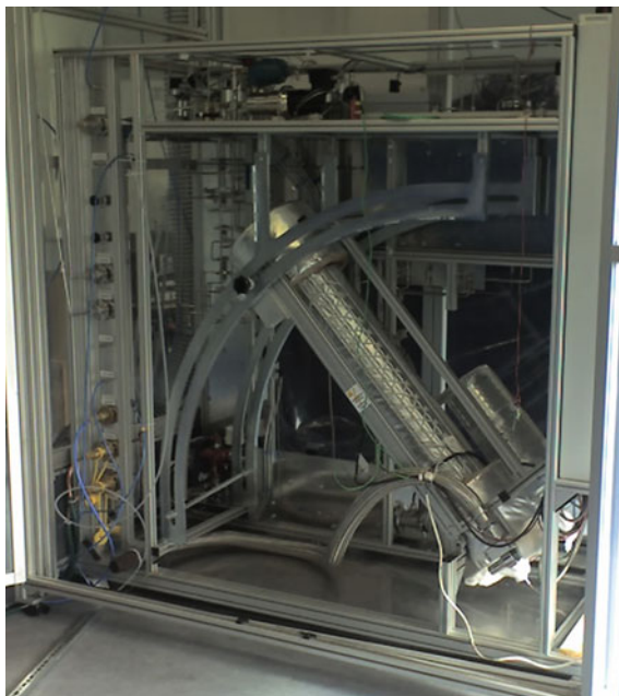
Fig. 9.5 The MPCP GmbH pilot plant for deep hydrodesulphurization of jet fuel. The adjustable reactor position is designated for simulations on board (reprinted from [7] with permission from Elsevier)
