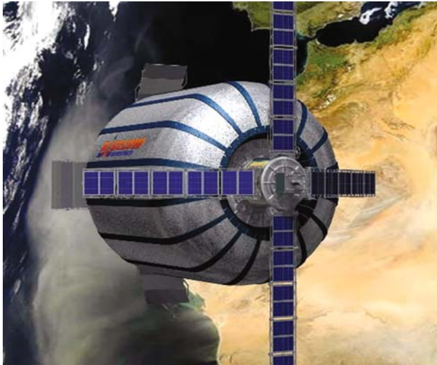
FIGURE 7.11. The Bigelow Aerospace Genesis II prototype space hotel module. Successfully launched in June 2007, the test-bed inflatable cylindrical structure is 4.4-m long and 2.5 m in diameter. By 2012 Bigelow Aerospace plans to offer a 4-week orbital trip, the price of the holiday coming in at about $500,000 a day.
