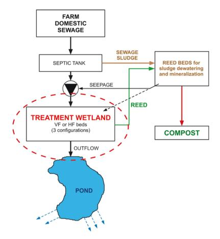
Fig. 9.1 The concept of sewage and sludge management for an individual household
