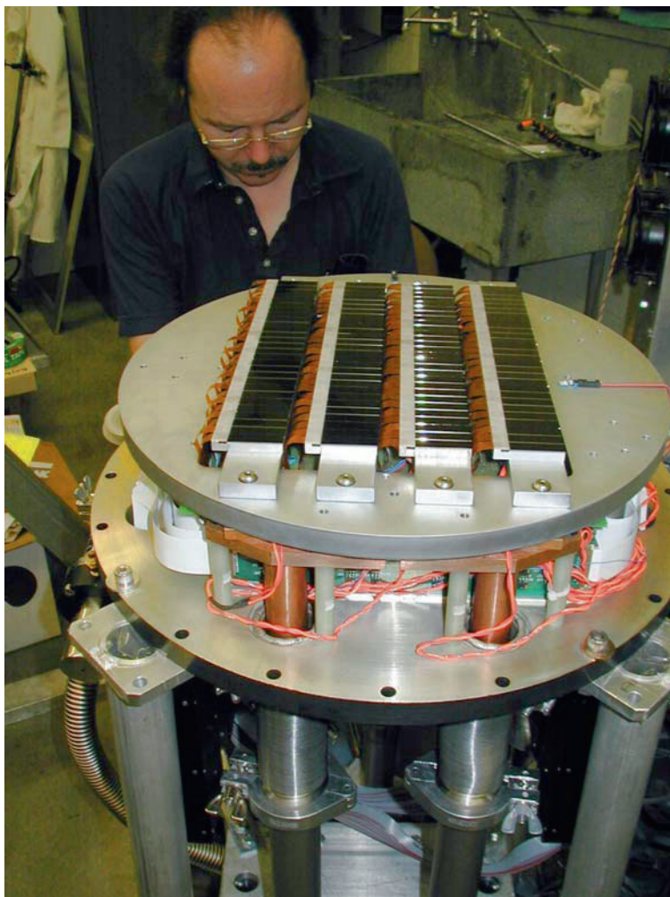
The QUEST camera with its rows of CCD detectors. In the background is electronics designer Mark Gebhard (David Rabinowitz)
