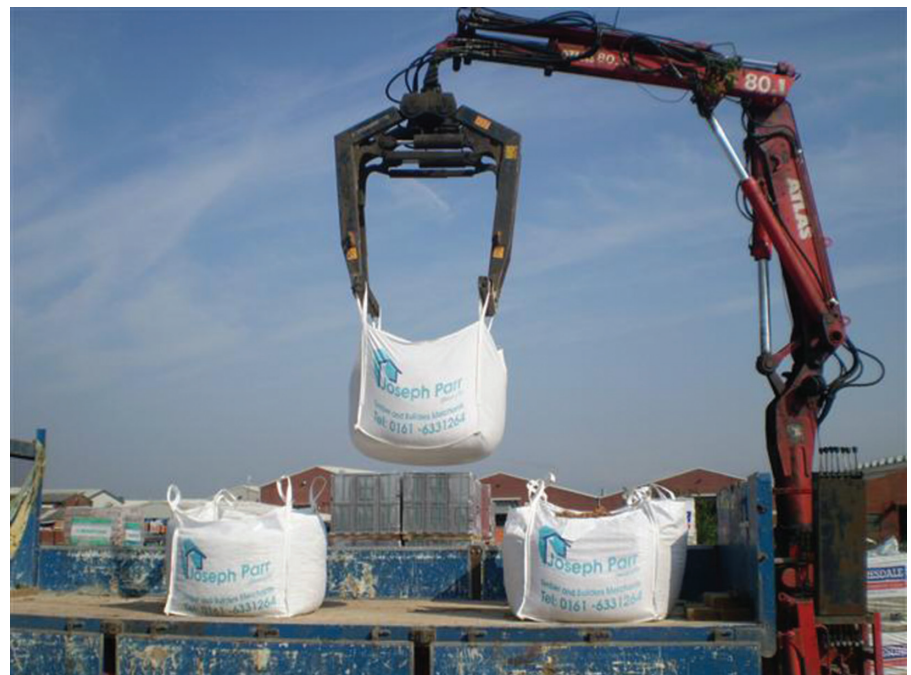
Figure 14.5 A crane moving bulk materials in large, reusable heavy-duty bulk bags from a truck for use in construction. (Photograph courtesy of Custom Packaging Products)
