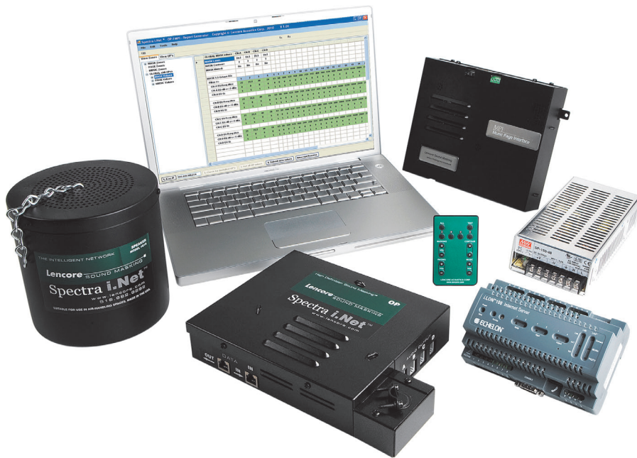
Figure 13.5 A networked sound-masking system manufactured by Lencore Acoustics Corporation includes digital signal processors, electronic noise generators, amplifiers, wiring, loudspeakers, controls, and other components to generate, amplify, distribute, and reproduce digitally synthesized and stabilized background sound masking to create speech privacy. (Photograph courtesy of Lencore Acoustics Corp. www.lencore.com )
