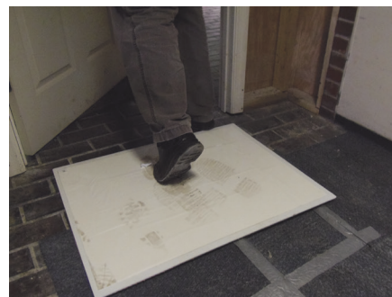
Figure 14.4 Sticky mats and walk-off mats are entrance control measures to help reduce contaminants entering into a clean area. (Photograph courtesy of D. Stephany)
