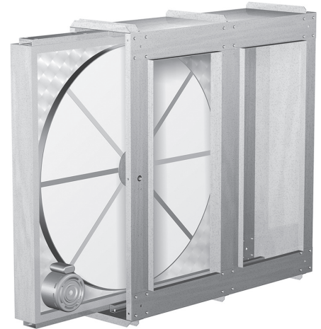
Figure 9.19 The ERV manufactured by Greenheck, Inc., houses a desiccant wheel that rotates between fresh and exhaust air streams, exchanging energy and humidity and providing enormous energy conservation benefits. (Photograph courtesy of Greenheck, Inc.)
