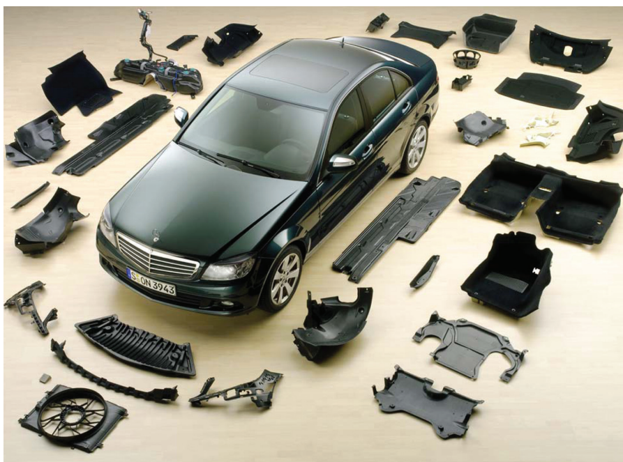
Figure 3.30 A Mercedes Benz can be quickly disassembled for end-of-vehicle life recycling. (Photograph courtesy of Mercedes Benz GmbH, Stuttgart, Germany)
