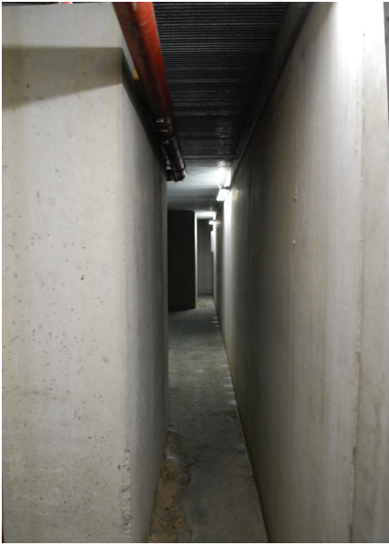
Figure 7.10 After entering the building through the outside air intake grilles, air flows through the earth canal, which cools the air via ground contact in summer and heats it in winter.
