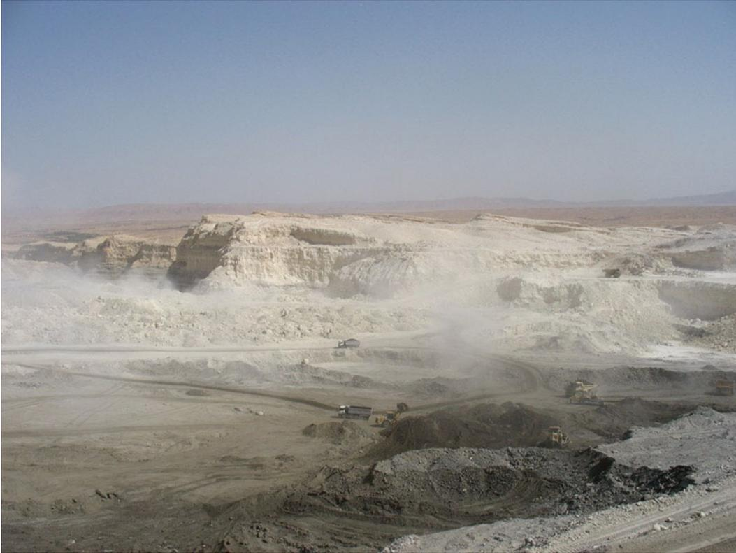
**Photo 10.3** Important sources of air pollution in opencast mining are motor transport and handling operations. The main component of atmospheric contamination is mineral dust. An
