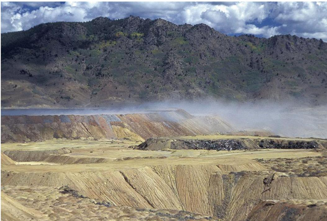
**Photo 10.4** One more source of air pollution in opencast mining is dust-forming surfaces (dumps, slopes, tailing dumps, etc.). The dust kicked up by the wind at a Yankee
