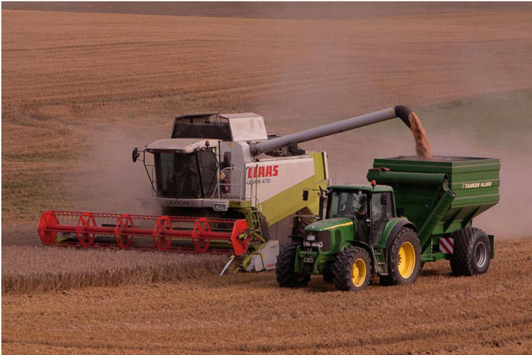
**Photo 11.5** The most environmentally important impact of plant growing is due to contact of soils with machinery. The ground is affected by the drive systems and operating parts of the agricultural equipment. By the end of fieldwork, only 10–15% of the agricultural land is not affected. The rest of the
