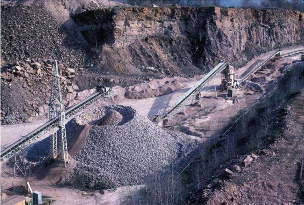
**Photo 9.21** The manufacture of goods from natural rock materials also is accompanied by dust discharges. The major manufacturing operations producing dust include (1) crushing, (2) cracking, (3) transfer to charging grid, (4) transportation, and (5)
