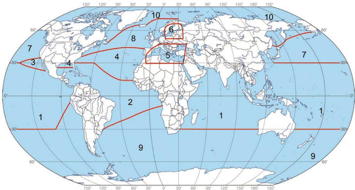
**Fig. 5.39** Areas of similar ship fouling (Marine fouling and its prevention 1952). Numbering of the areas in arbitrary, and is not intended to indicate relative fouling (Reproduced with permission of U.S. Naval Institute, Annapolis, Maryland)
