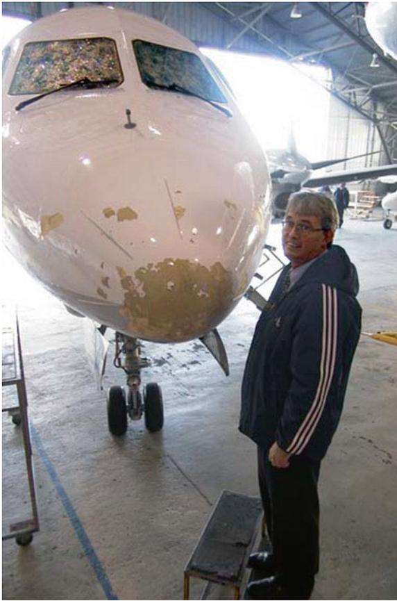
**Photo 3.27** Of all kinds of transportation, aviation is affected the most by hail. Hail blows break windshields and the surfaces of airplanes. They cause flight performance to deteriorate. This photo shows a Saab-340 airplane with windowpanes damaged by hail during a flight from Wellington to Napier. The pilot had to land at the airport of Palmerston North, North Island, New Zealand (Photo credit: *Manawatu Standard* newspaper, Palmerston North, New Zealand, June 2000)
