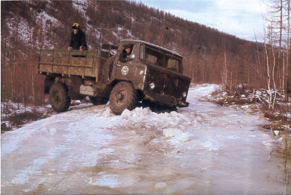
**Photo 2.25** Aufeises make roads slippery, which increases the number of road accidents. When an aufeis is not yet frozen on the top, cars bog down and freeze into ice if they stop. The photo
