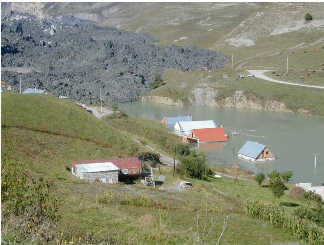
**Photo 4.40** The impact of the Kolka surging glacier on dwellings during the surge of 20 September 2002 resulted in both destruction of buildings due to dynamic impact of ice and debris and their further inundation by melted ice. The photo shows a
