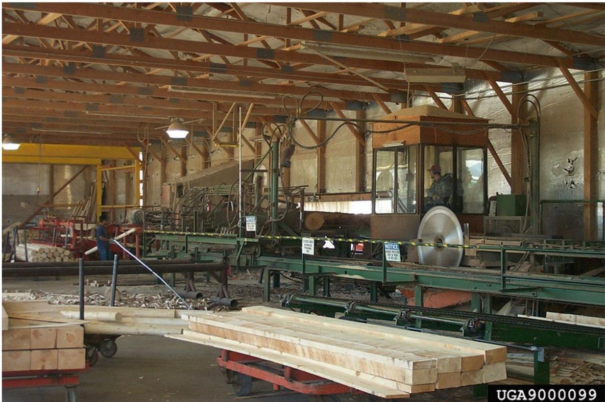
**Photo 9.23** Mechanical processing of wood is generally based on four working operations: (1) sawing, (2) planing, (3) drilling, and (4) polishing. As a result, sawn goods are produced that are used in construction, and manufacture of furniture, finishing
