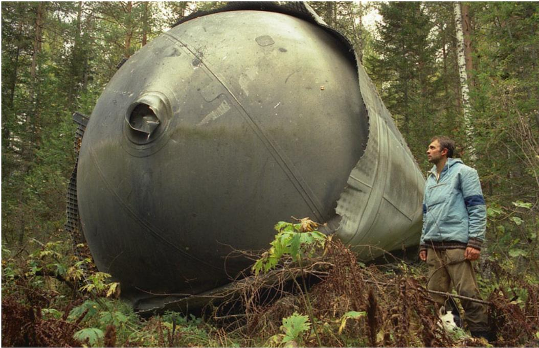
**Photo 13.30** The second stages of carrier rockets separate at altitudes of 140–160 km. Due to heating in the atmosphere, the fuel explodes when the stage is 25–30 km above sea level. Fragments fall to the ground, covering a large area. The fuel tank
