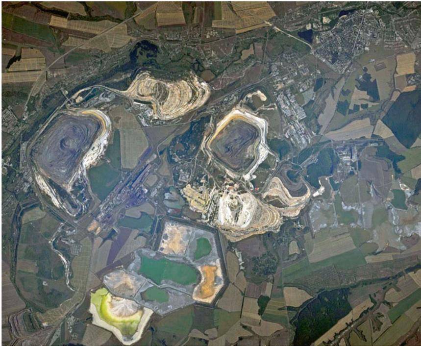
**Photo 10.1** An opencast operation is a powerful factor in relief transformation. The photo shows the Lebedinsky mining processing plant (Kursk magnetic anomaly, Russia). The depth of the open pit is 450 m, and its dimensions are 4 by 5 km. Annually, about 50 million cubic metres of mined rock is car-
