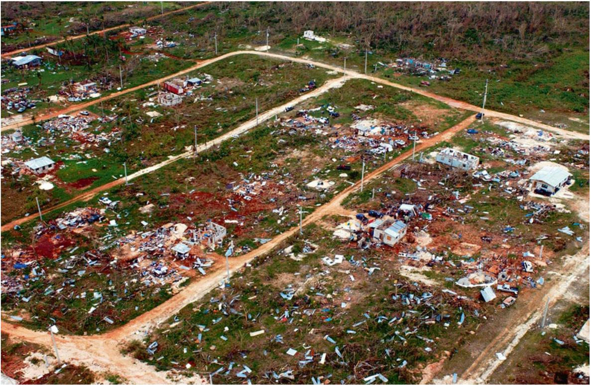
**Photo 3.3** The impacts of hurricanes on dwellings and industrial structures are caused, in particular, by strong wind. This aerial photo shows the extensive damage on Guam (Honolulu
