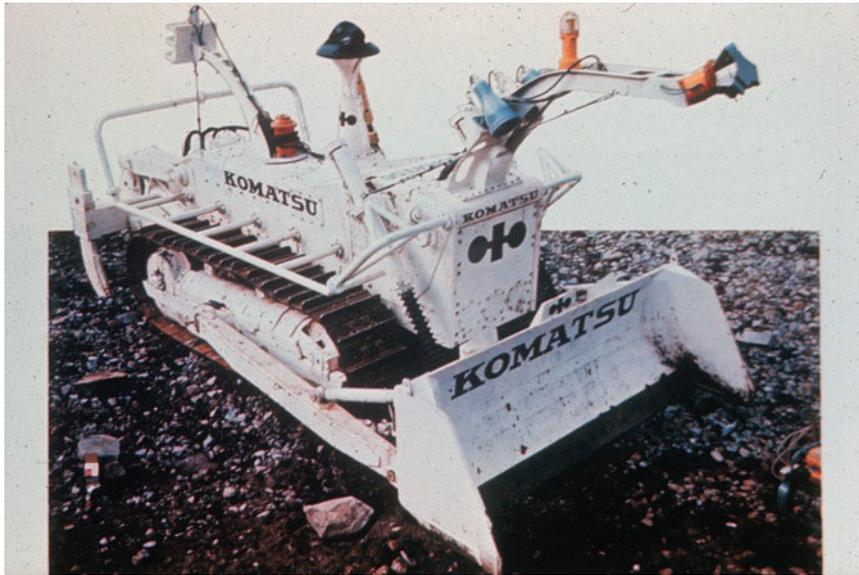
**Photo 12.11** In the process of building pipelines in the open sea, they are placed on the bottom fixed with anchorages (concrete slabs, blocks, etc.). If a pipeline must be laid deeper, ditches
