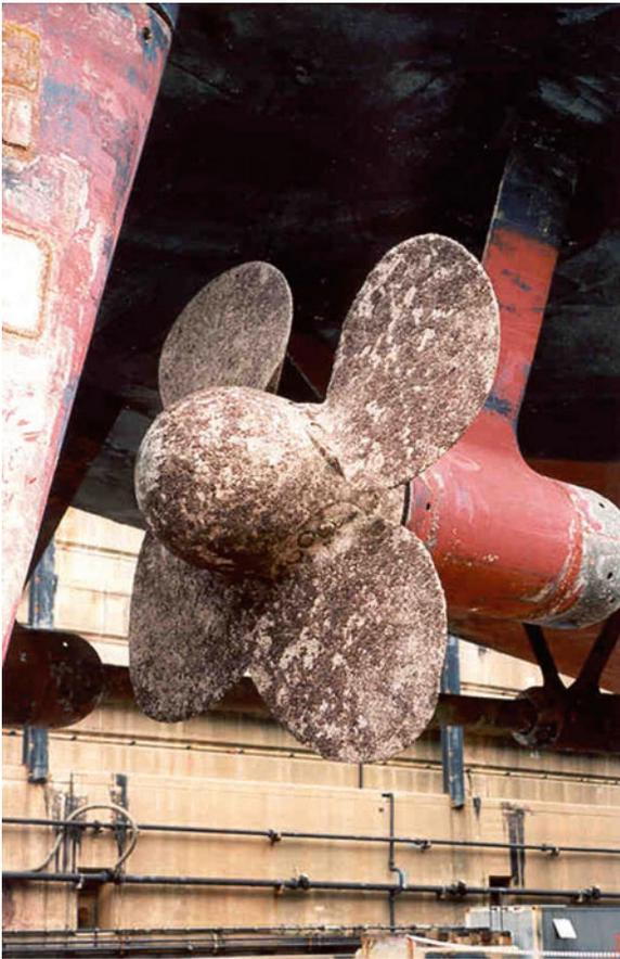
**Photo 5.121** Hull fouling is not the only reason for reductions in propulsive quality. Propeller fouling also leads to increases in fuel consumption. The photo shows a fouled propeller in Australia (Photo credit: Defence Science and Technology Organisation, Australia)
