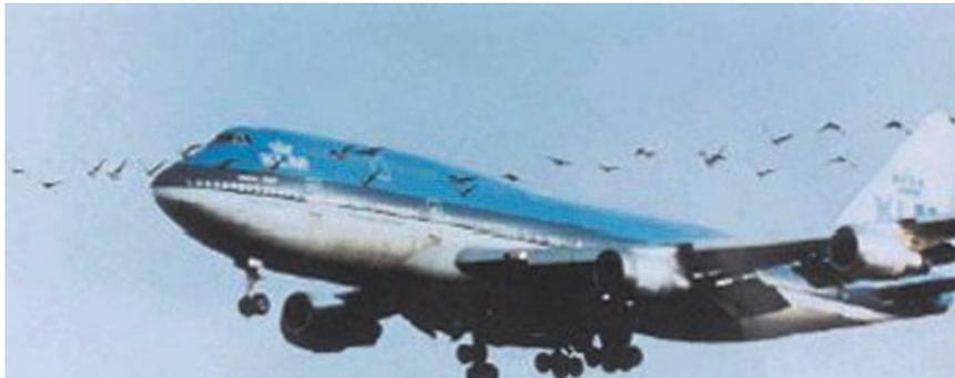
**Photo 5.115** With an aircraft speed of 555 km/h, a collision with a Canada goose (*Branta canadensis*; weight 6.8 kg) yields a force of 37,200 kg. The #1 engine on this KLM B-747 suffered an
