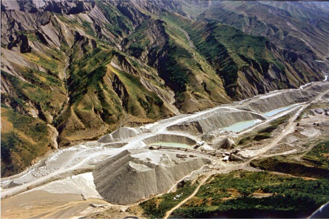
**Photo 10.12** For development of river placers, cleaning the surface of vegetation, development mining (removal of the upper non-productive stratum), watering, and production (extraction of the commercial component from the productive stratum) are
