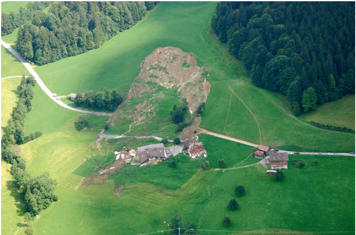
**Photo 2.14** The impacts of landslides on a structure depend on the location of the object, which can be situated either within the landslide area or underneath it. The first situation is illustrated in
