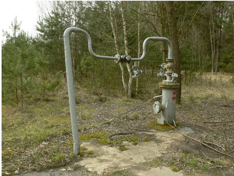
**Photo 10.15** During *in situ* leaching, the leaching solutions are supplied through wells to the underground ore body; then the solutions, saturated with metal, are pumped out to the surface. Further along, the metal is extracted from the solution. Major environmen-
