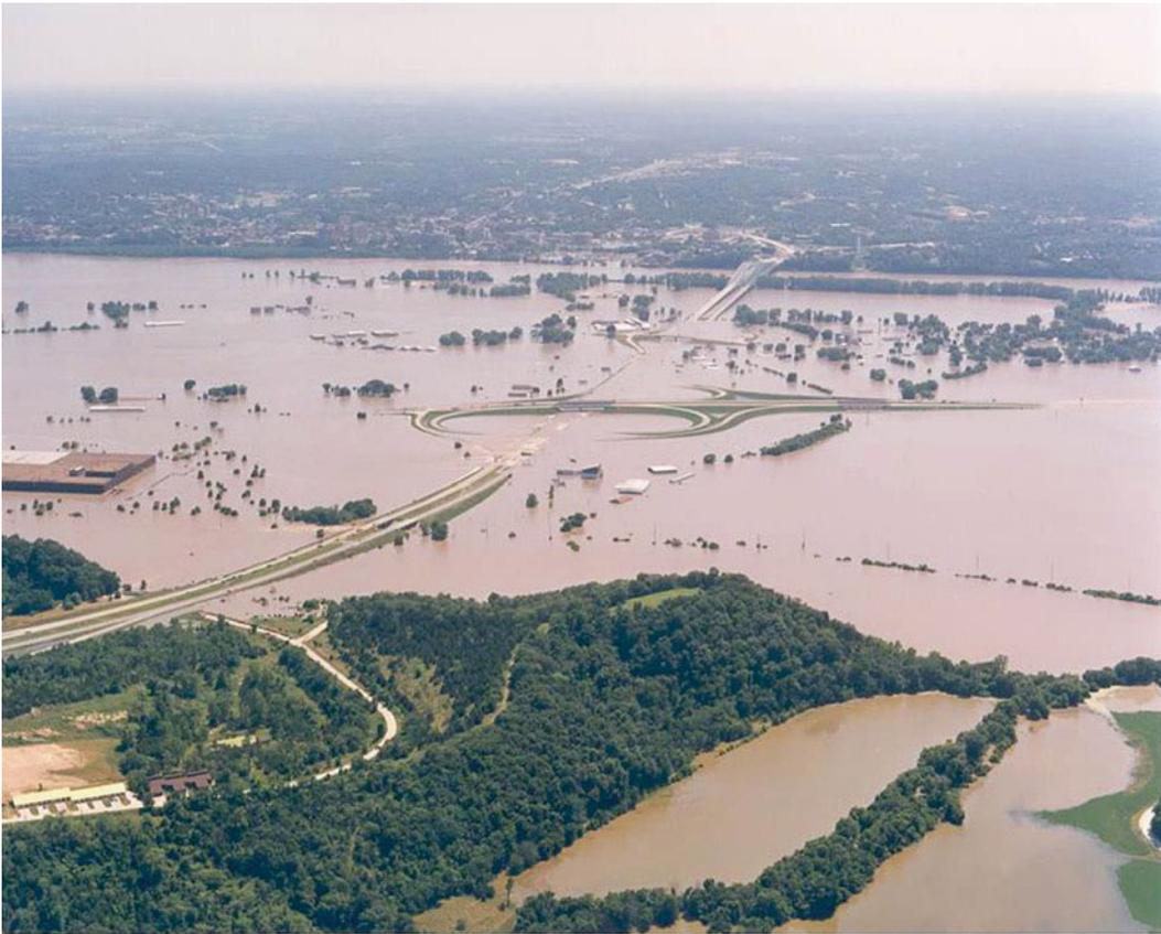
**Photo 4.3** Nevertheless, if water depths exceed a certain threshold, car traffic stops and earthworks and roadbeds are damaged. The photo shows the Missouri River flooding in the
