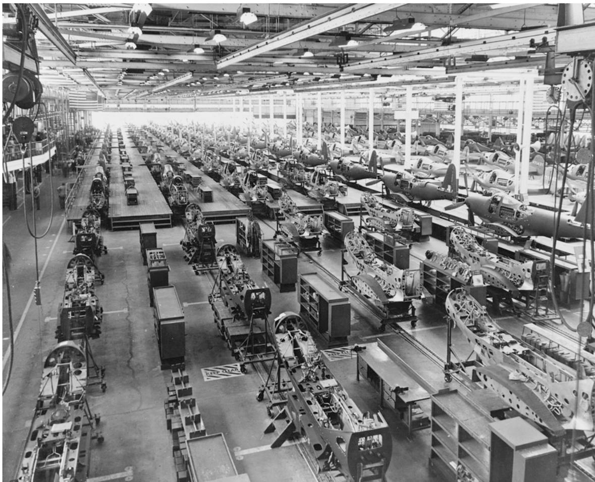
**Photo 9.16** There are two types of assembling works: (1) stationary (all components and units are fed to one place, the assembly stand) and (2) mobile (yet-to-be-assembled units move successively through all stands). The photo shows the assembly
