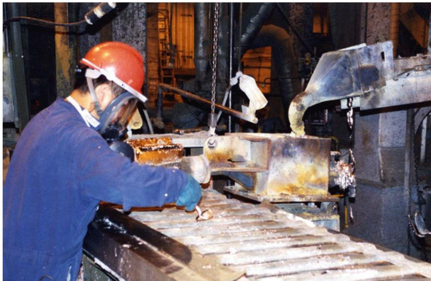
**Photo 9.19** In battery factories, the air is contaminated with dust containing lead, nickel, cadmium, arsenic, bismuth, antimony, and tin. The photo shows a worker who is ladling molten recycled lead into billets in a lead-acid battery recovery
