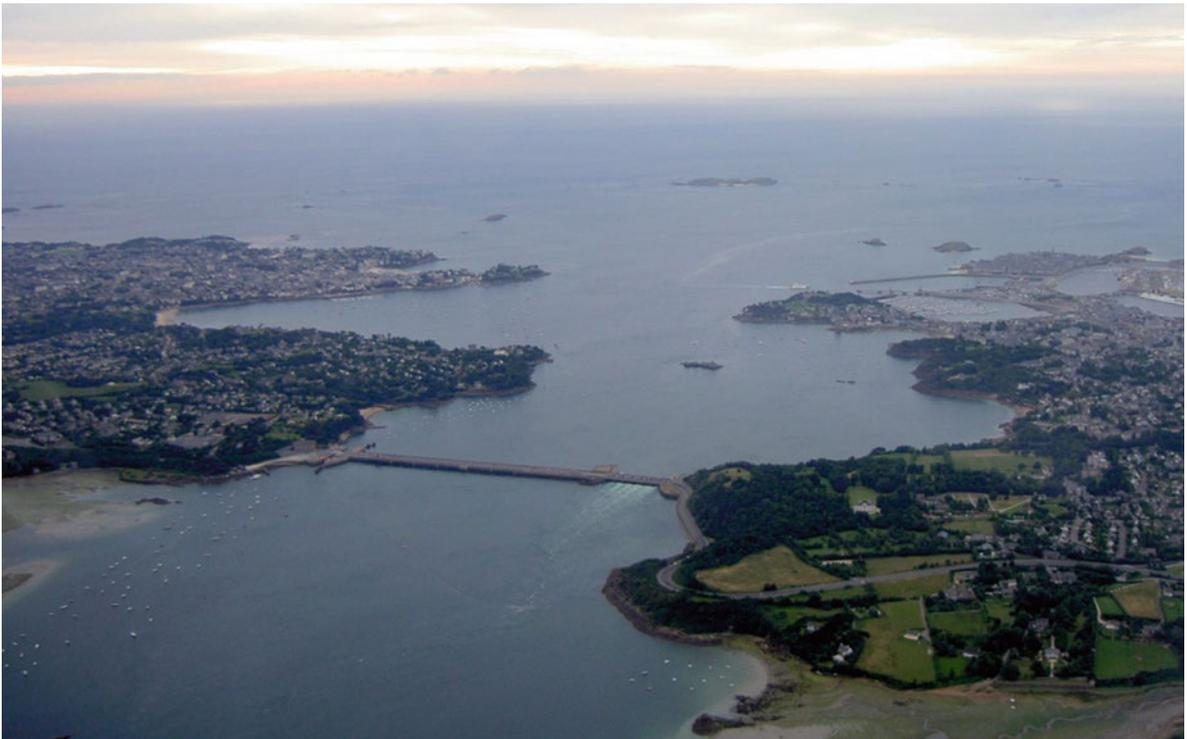
**Photo 8.22** The major influencing factor of the effect of tidal hydroelectric stations on the environment is a reduction in the natural water exchange of the cut-off part of water area with the sea. First of all, this influences hydrobionts. The La Rance tidal power plant shown here, off the Brittany coast
