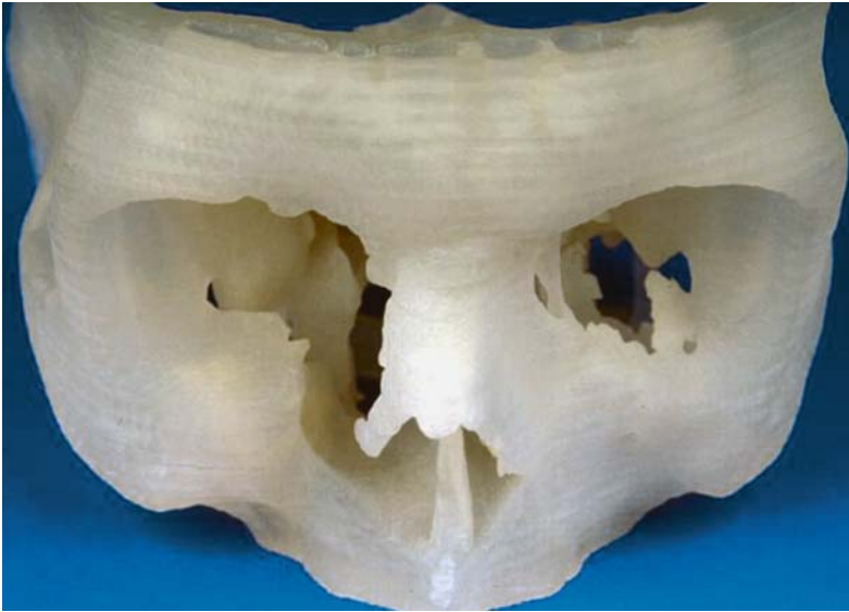
Fig. 16. Stereolithographic model of the naso-orbitoethmoid region. The frequent appearance of pseudo-foramina in areas of very thin bone is a serious hindrance to planning, especially in orbital wall reconstructions
