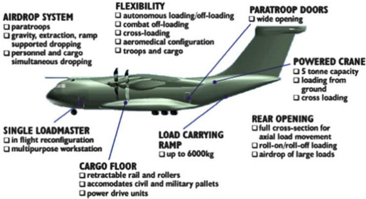
**Fig. 12.32** The main characteristics of the A400M (Picture from the Airbus Military Company website: [airbusmilitary.com](http://airbusmilitary.com))
