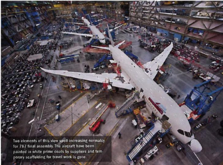
**Fig. 6.22** The final assembly line (FAL) of the B787 Dreamliner (Photo Boeing published in *Aviation Week and Space Technology*, (2011), June 20, p. 86)
