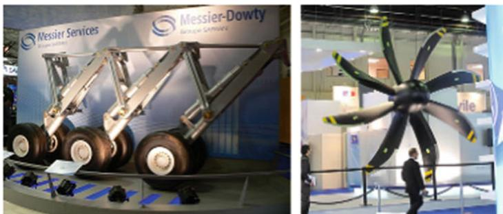
**Fig. 12.34** A400M landing gear (by Messier Dowty) displayed at Paris Air Show in 2007, and the A400M propeller (Hamilton Sundstrand) at the Paris Air Show in 2009 (Picture from the Airbus Military Company website: [airbusmilitary.com](http://airbusmilitary.com))
