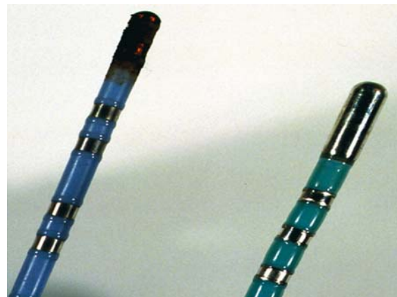
Fig. 2.2 Charring with 8 mm tip electrode catheters
