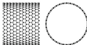
Fig. 13.4 Lateral (aside) and cross-sectional (across) images of hexagonal single-wall BN nanotubes with different chiralities and diameters
