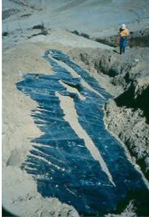
and Canyon D. Figure 13.1 shows the tear observed in the Canyon D liner system after the earthquake.
