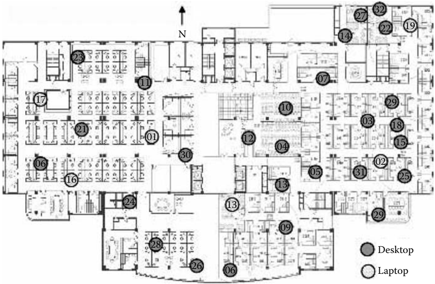
Figure 3.13 Our testbed, consisting of 32 nodes placed in fixed locations inside an office building.
