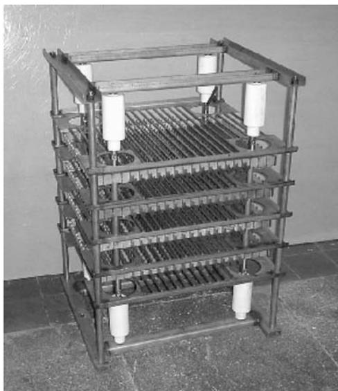
*Figure 4.* Pulsed corona block electrode structure
