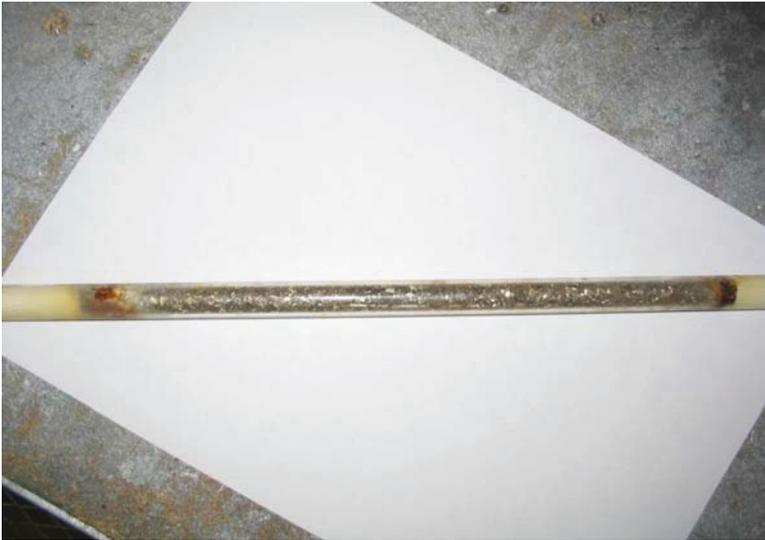
*Figure 9.* Electrodes condition of DBD optimized for air with natural humidity after 1 year nonstop operation. We can see no deposition of acid on the surface of electrodes
