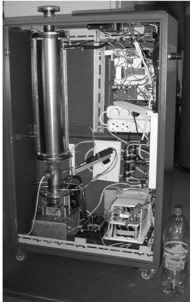
*Figure 12.* Plasma converter of hydrocarbons with 0.5–5 kW (2,45 GHz) power. Productivity level about 10 standard meter cubic of syngas per hour
