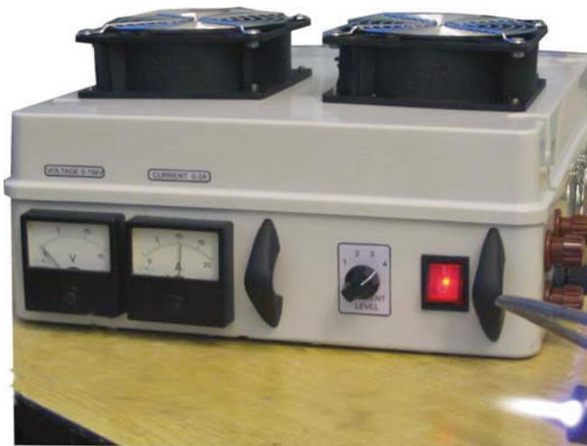
Figure 3. DC power supplies for different kinds of arc and glow discharge applications
