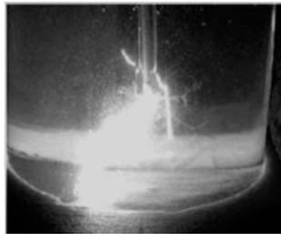
*Figure 9.* Electro-hydraulic spark discharge in water
