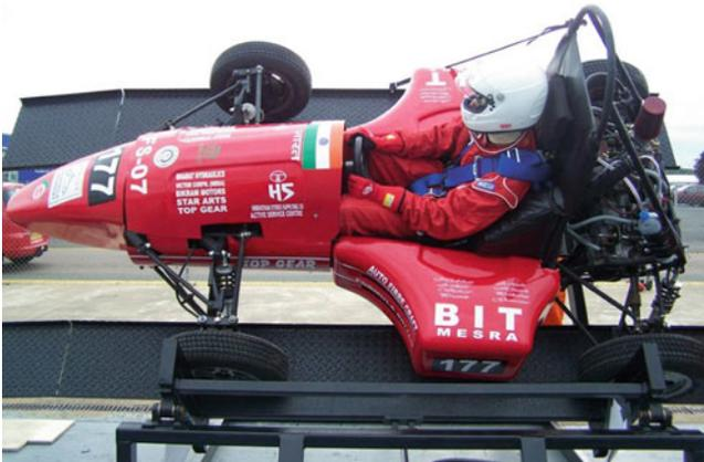
Fig. 9.4 Formula student car body developed by AFC in GFRP by hand layup technique
