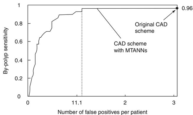
**Fig. 12.6** The FROC curve that shows the overall performance of the mixture of expert 3D MTANNs when it was applied to the entire database of 27 polyps and 224 FPs. The FROC curve indicates that the mixture of expert 3D MTANNs yielded a reduction of 63% of nonpolyps (FPs) without removal of any true positives, i.e., it achieved 100% classification performance
