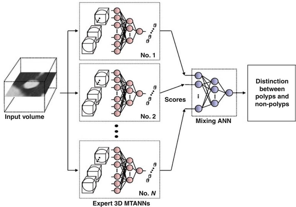
**Fig. 12.4** A mixture of expert 3D MTANNs for distinguishing lesions (polypoid and flat lesions) from various types of FPs. Each expert 3D MTANN consists of a linear-output regression ANN model. Each MTANN is an expert for distinguishing lesions from a specific type of FP. The outputs of the expert 3D MTANNs are combined with a mixing ANN so that the mixture of expert 3D MTANNs can remove various types of nonlesions
