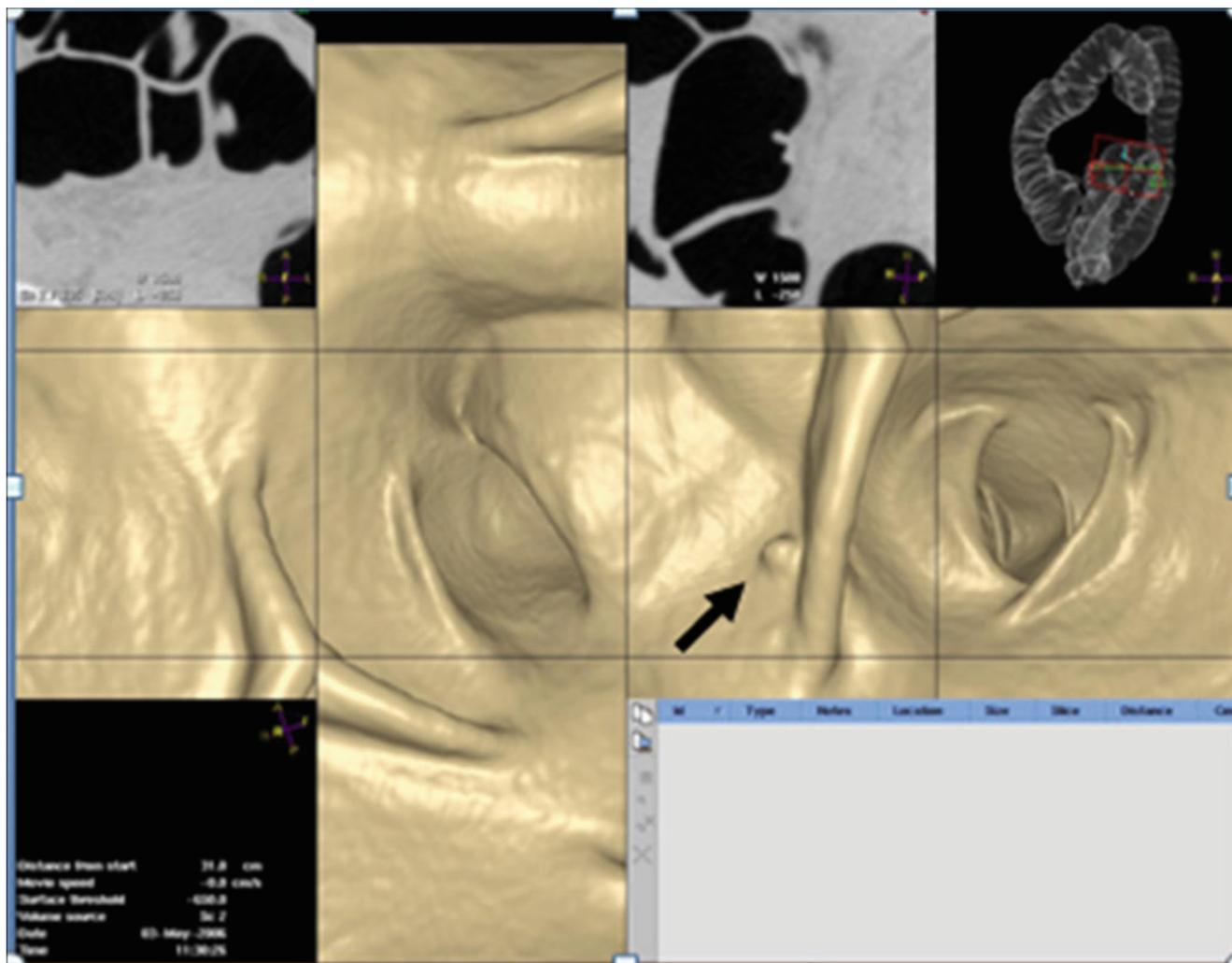
**Fig. 8.22** Unfolded cube projection. This display method opens (“unfolds”) the segment being evaluated from the center of an imaginary cube. The six images of the unfolded cube include the forward (F) and
