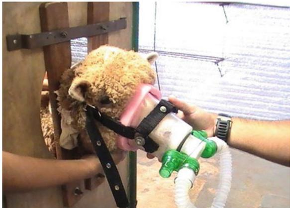
**Fig. 8.4** Facial mask used to evaluate the metabolic heat production of chickens (Nascimento et al. 2011)
