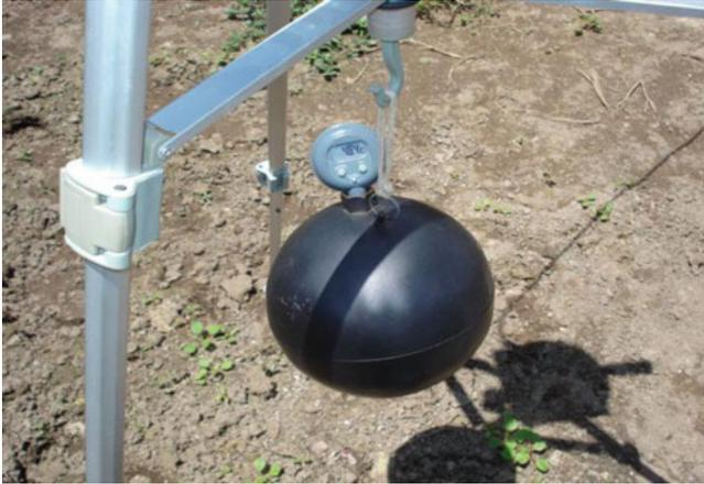
**Fig. 1.3** *Black globe* used to evaluate radiant heat load. Over the globe, there is the display of the digital thermometer that was introduced for the determination of the globe temperature,  $T_g$
