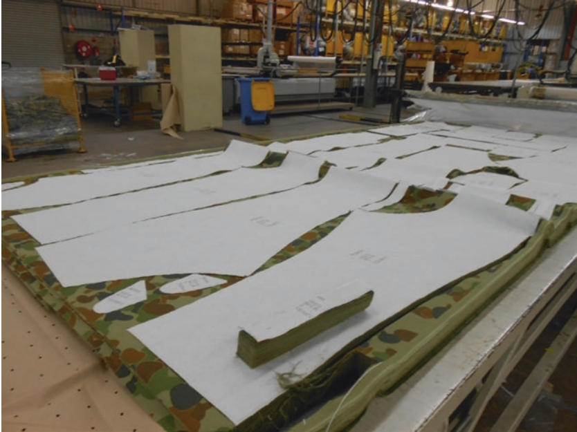
Fig. 7.6 Multiple layer uniform pattern pieces cut on the Gerber S90 cutting machine at Australian Defence Apparel Pty. Ltd., Bendigo, Victoria. Source: Author's photo. Note the many layers of the camouflage combat uniform cut at once
