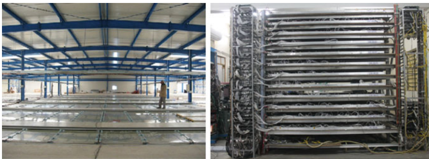
Fig. 4 6700 \text{ m}^2 RPC carpet array of ARGO-YBJ experiment (left), INO's 2 \text{ m} \times 2 \text{ m} RPC detector stack (right)
