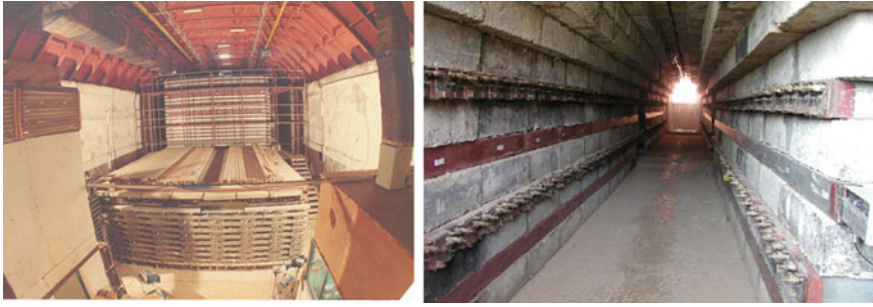
Fig. 2 Proportional counters in the KGF proton decay experiments (left) and in the Grapes-3 experiment in Ooty
