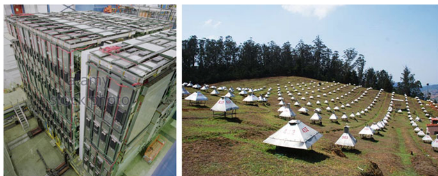
Fig. 3 D0 muon scintillator detector (left), scintillator based timing detectors of Grapes-3 experiment (right)
