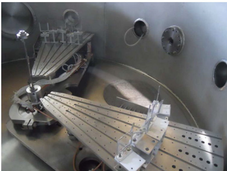
Fig. 3 PET films mounted on aluminum holders and placed on two movable arms inside the general purpose scattering chamber
