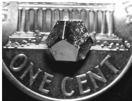
FIGURE 8.4. A quasicrystal of a scandium-zinc alloy displays icosahedral symmetry. Image courtesy of Paul C. Canfield at Ames Laboratory and Department of Physics and Astronomy, Iowa State University.
