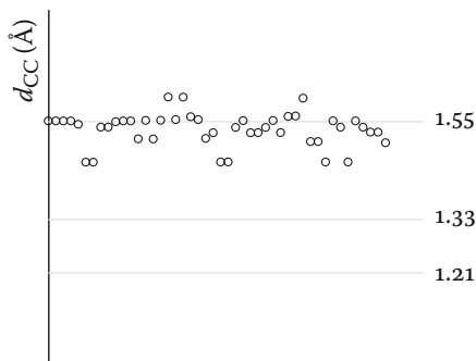
FIGURE 8.11. After three minimization steps, the C-C distances have relaxed somewhat from the typical 1.55 Å distance characteristic of a carbon-carbon single bond.
