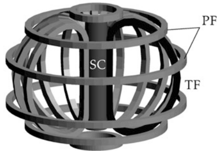
FIGURE 11.13. Schematically, the main magnets of ITER consist of 18 toroidal field (TF) magnets that generate an azimuthal field. Several are not displayed here to visualize the central solenoid (SC). The six poloidal field (PF) magnets form continuous rings around the toroidal magnets.
