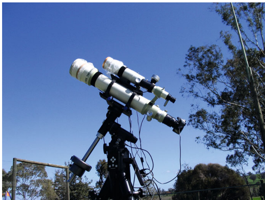
Fig. 5.12. Refracting telescopes mounted on an equatorial mount. Set up for photography. (JW).
