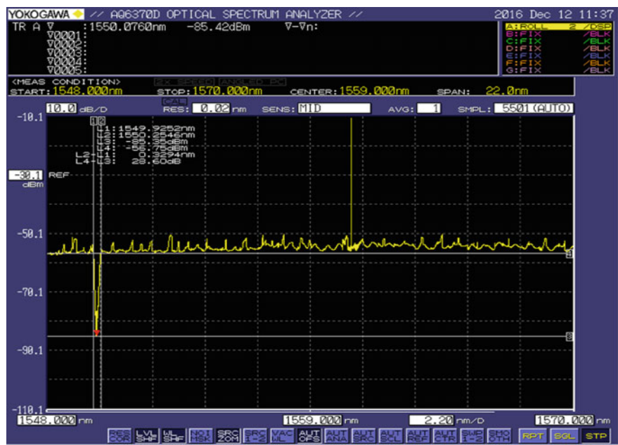
Fig. 5.27 FBG and NCF spectrum in H 2 O at 90 °C
