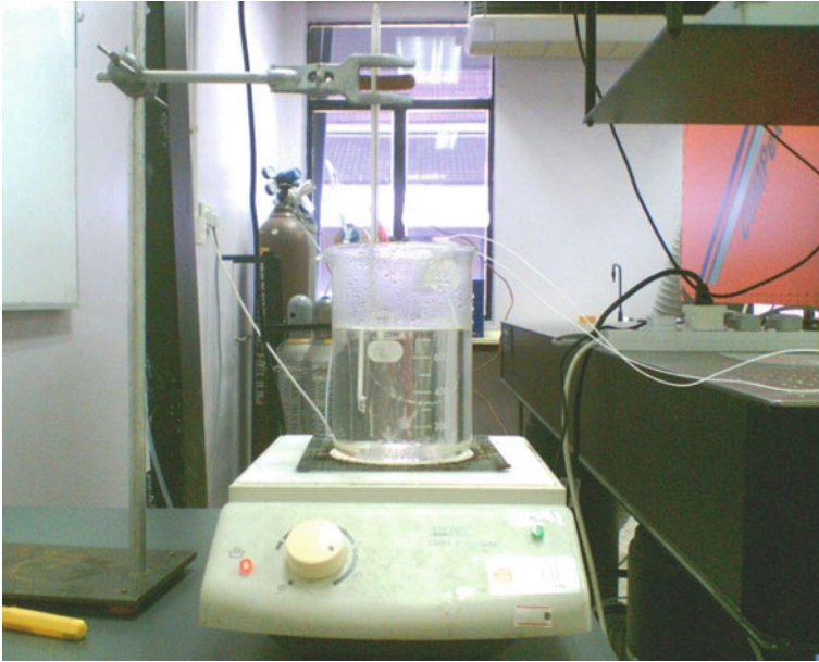
Fig. 4.3 Photograph of the experimental setup for temperature measurement in liquid
