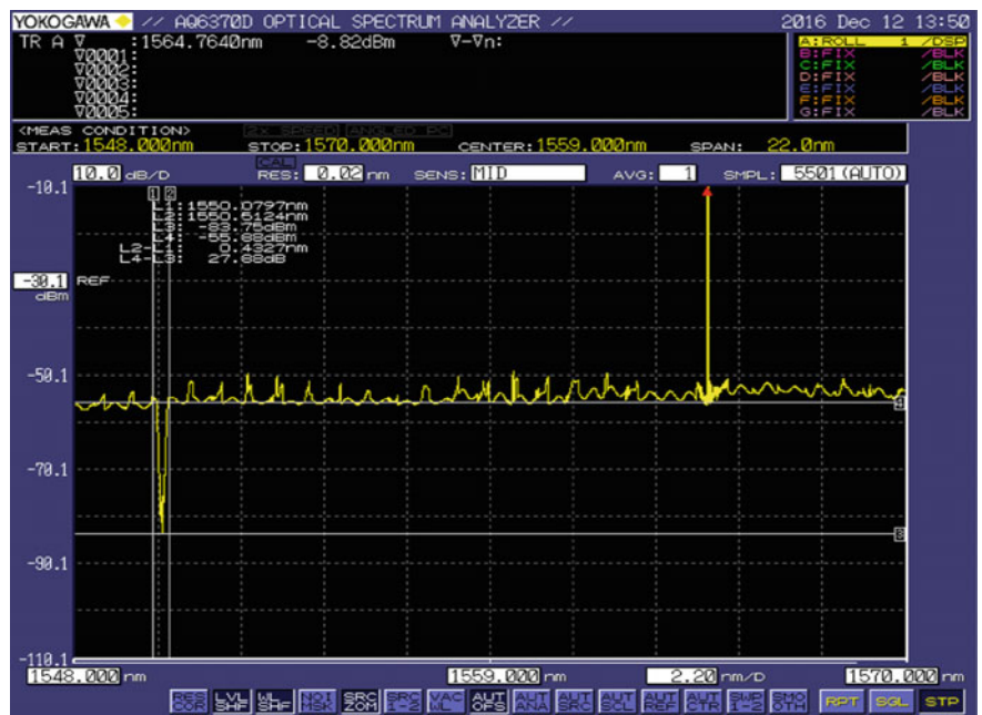
Fig. 5.29 FBG and NCF spectrum in NaOH solution at 90 °C
