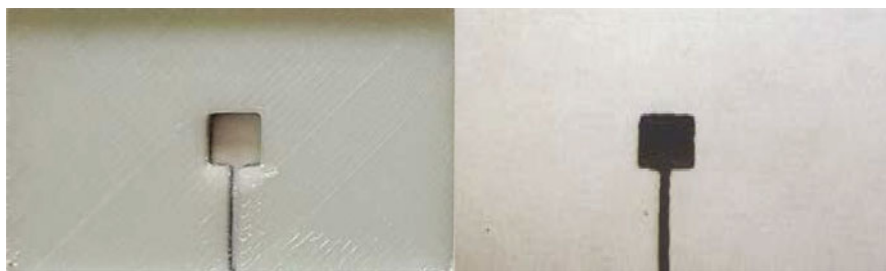
Fig. 12.1 Mask and electrode deposited on glass
