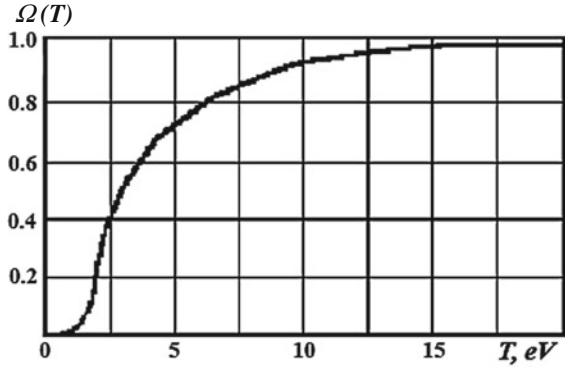
Fig. 7.11 Dependence of fraction of the arc radiation energy absorbed by the hydrogen versus arc temperature [26]
