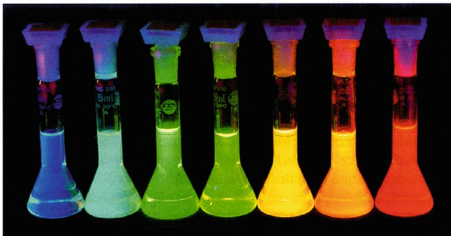
**Fig. 7** Size-dependent change of the emission colour of colloidal solutions of CdSe/ZnS core-shell nanocrystals. The particles with the smallest ( $\sim 1.7$  nm) CdSe core emit blue; the particles with the largest ( $\sim 5$  nm) core emit red. Reprinted from [143], Copyright 2004, with permission from John Wiley and Sons
