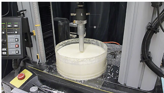
Fig. 4.1 Speed-controlled impact experiment. Image showing how the Instron 5586 materials testing device pushes a metal rod into the surface of a cornstarch and water suspension at a constant velocity v_0 while simultaneously recording its instantaneous position z_r and the force exerted on it F_r . The suspension is characterized by its packing fraction \phi_0 , viscosity \eta , and fill height H . With the 500 N force transducer used with the Instron in these experiments, we had a force resolution of \sim 2 \times 10^{-3} N and a displacement resolution of 100 \mu\text{m} . Image of the actual experiment
