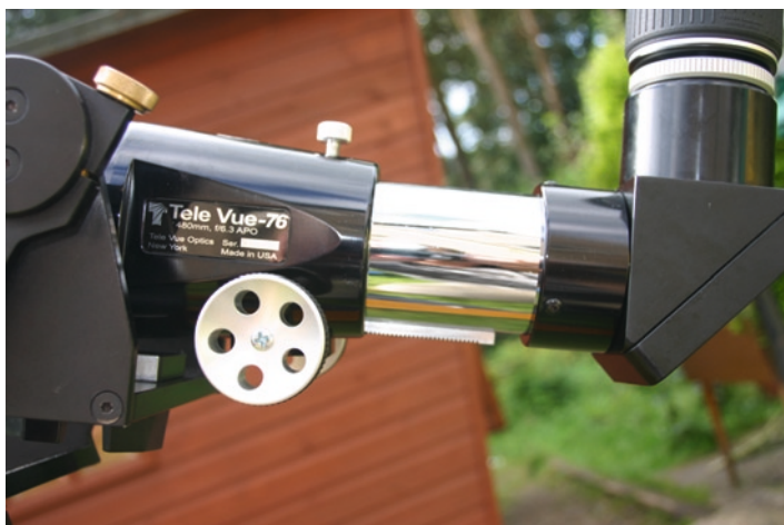
An exceptional rack and pinion on the TeleVue 76 (Image by the author)
