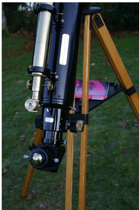
The brass finder and Baader Steeltrack focuser on the Skylight F/15
