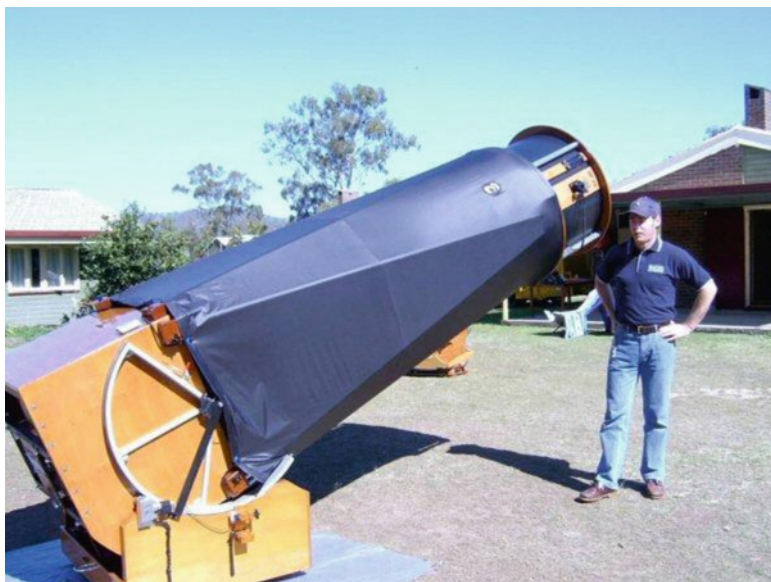
Fig. 8.6. The SDM 30-inch f/4.8 Obsession-like Dob (Image credit: SDM Telescopes).
