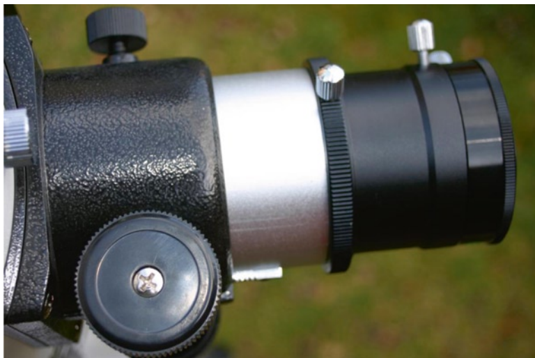
Fig. 3.15. The simple but effective rack and pinion focuser on the Skyliner 150P (Image by the author).
