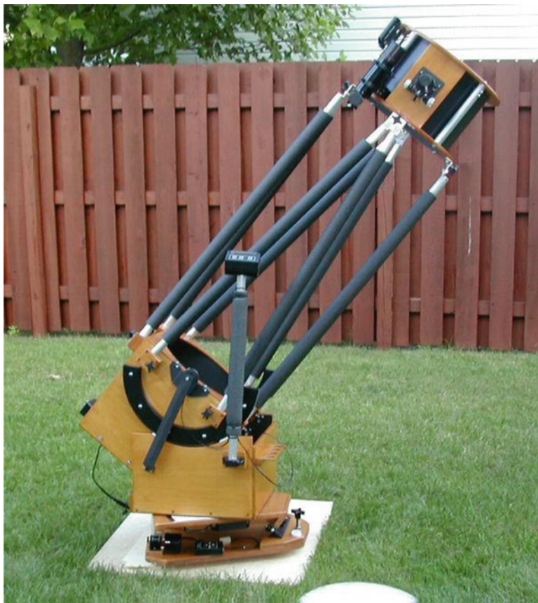
Fig. 9.7. A 12.5-inch truss tube Dob astride an equatorial platform (Image credit: Ron Klein).
