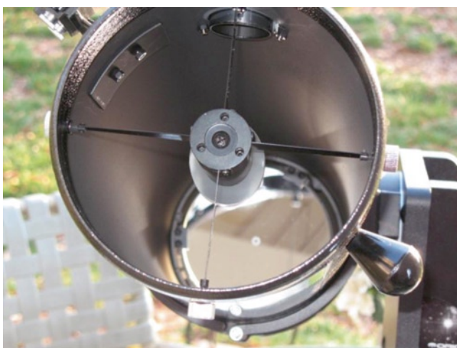
Fig. 3.11. The secondary is held in a fully adjustable holder by a four-vane spider (Image credit: Scott Holland).
