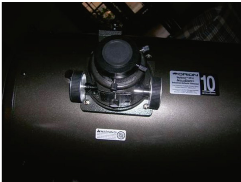
Fig. 4.7. The basic but functional Crayford focuser on the Orion XT 10 (Image credit: Javier Medrano).
