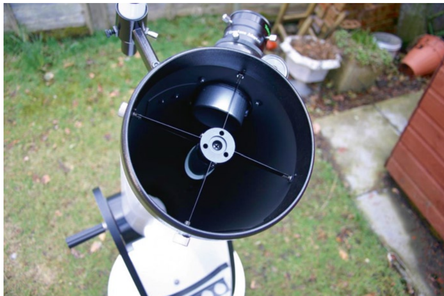
Fig. 3.18. The central obstruction due to secondary is a respectable 31 mm (1.25 inches).
