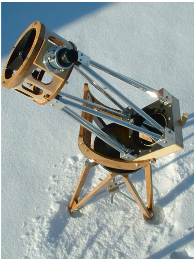
Fig. 7.5. Star Gazer Steve's elegant 6-inch f/5 truss tube Dob (Image credit: Patrick Dodson).
