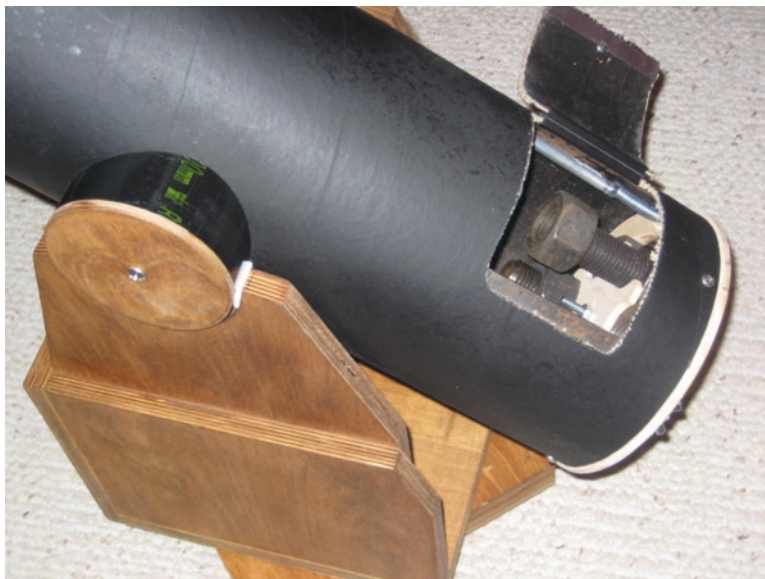
Fig. 5.6. The completed tube base together with balancing weights (Image credit: Vic Graham).
