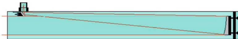
Fig. 5.12. Optical design of the DGM OA Newtonians. Note its totally unobstructed optics (Image credit: DGM Optics).
