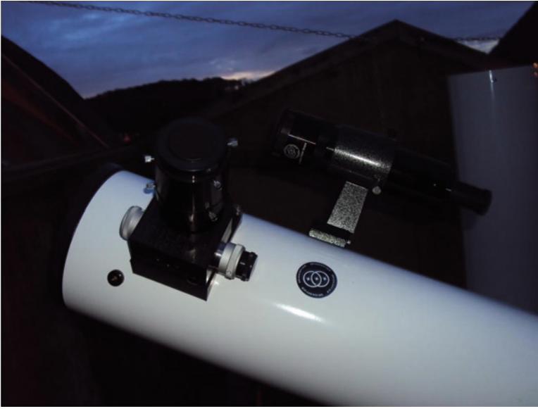
Fig. 5.9. The high-quality Crayford focuser on the Orion planetary Dob (Image credit: Pat Conlon).
