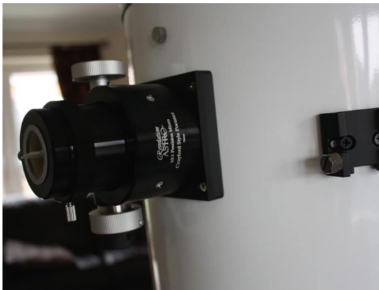
Fig. 6.7. The quality Crayford focuser on the Revelation 12-inch Dob (Image credit: Andy Sheen).
