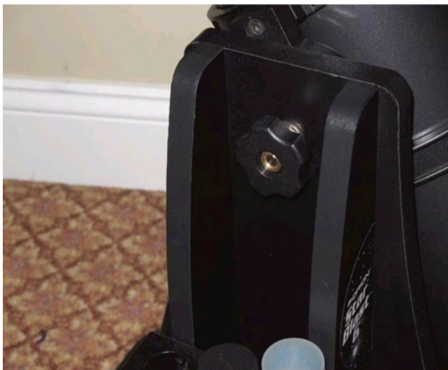
Fig. 3.7. The adjustable friction knob on the Starblast 6 mount (Image credit: Scott Holland).
