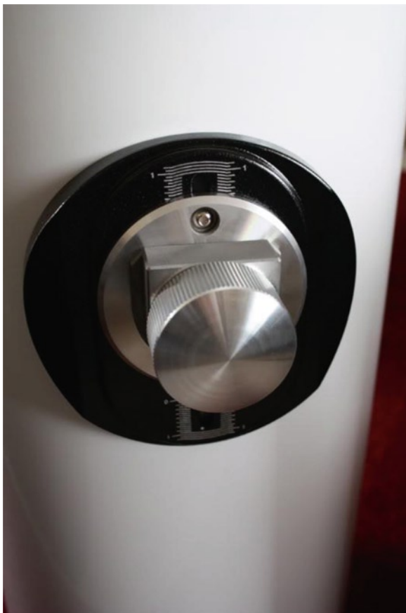
Fig. 6.5. The large knobs used to affix the OTA to the mount (Image credit: Andy Sheen).
