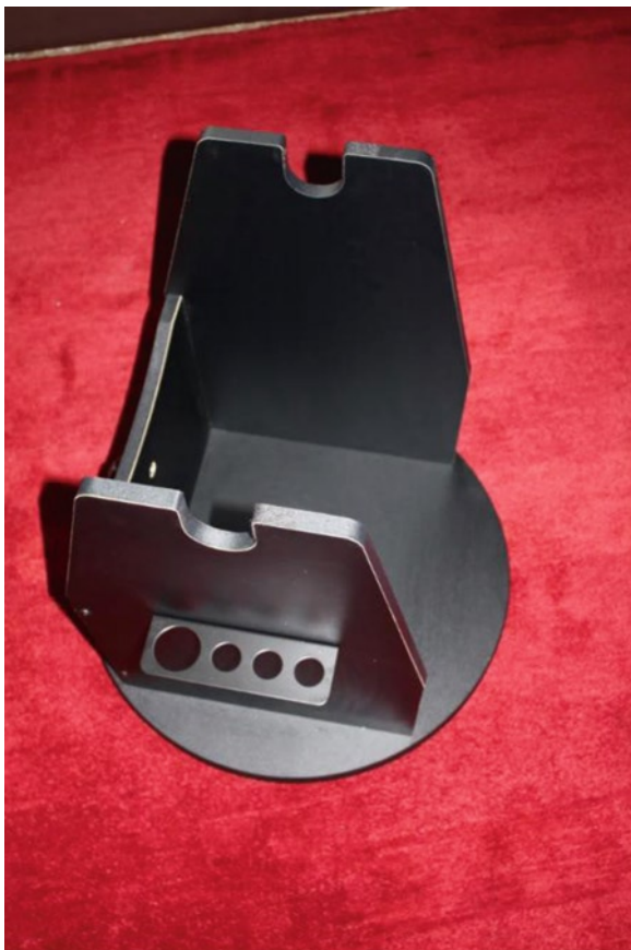
Fig. 6.4. The completed Lazy Suzan base (Image credit: Andy Sheen).
