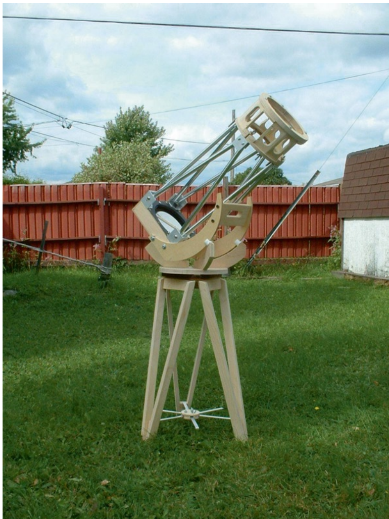
Fig. 7.6. Star Gazer Steve's 6-inch f/5 truss tube atop its elegant tripod (Image credit: Patrick Dodson).
