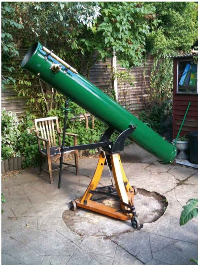
Fig. 7.10. A refurbished Calver reflector on an alt-az mount (Image credit: Robert Katz).
