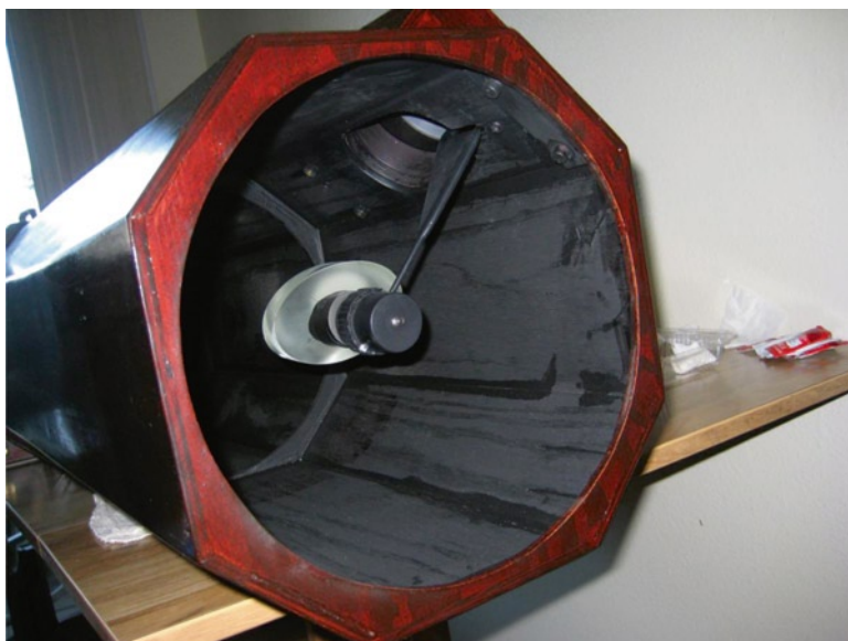
Fig. 7.12. The single vane securing the secondary mirror (Image credit: Norm Butler).
