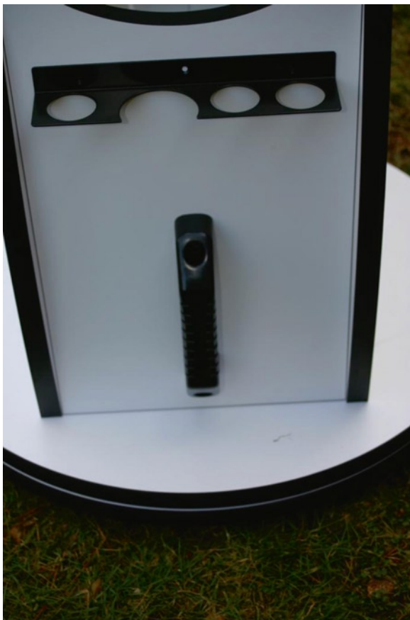
Fig. 3.16. Nice touches, like the carry handle and eyepiece caddy, make both moving the 'scope and observing with it a breeze (Image by the author).
