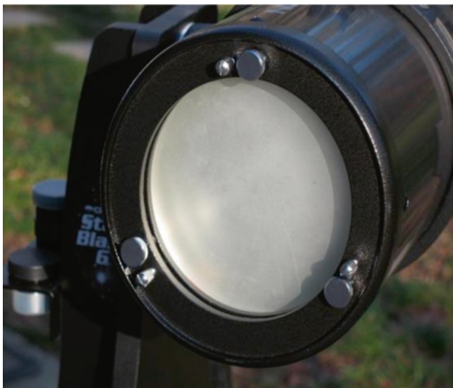
Fig. 3.9. The primary mirror cell has three spring loaded collimation knobs and three locking screws (Image credit: Scott Holland).
