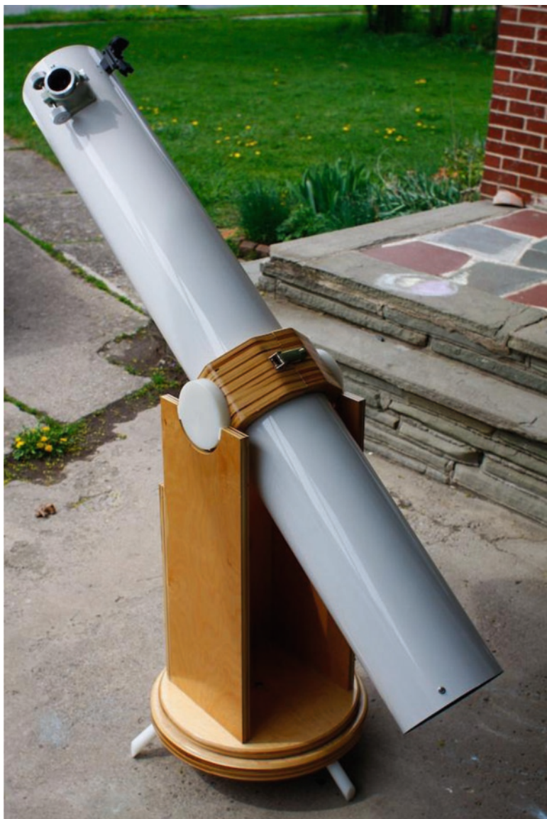
Fig. 5.11. The DGM OA 5.5 inch on a simple Dobsonian-style mount (Image credit: Doug Reilly).
