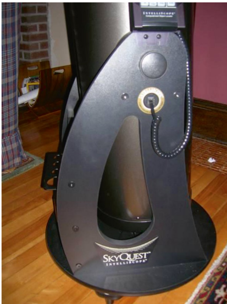
Fig. 4.8. A close up of the encoders that enable “PushTo” capability on the Orion XT10 (Image credit: Javier Medrano).
