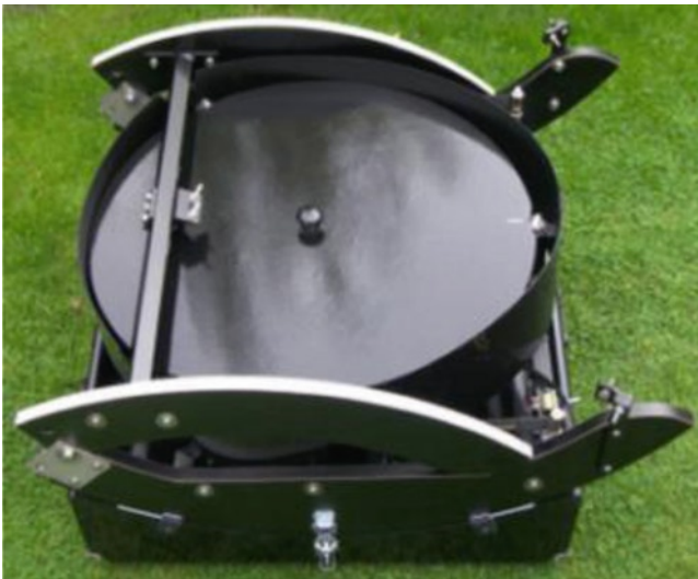
Fig. 8.4. The dismantled telescope with altitude bearings folded (Image credit: David Lukehurst).
