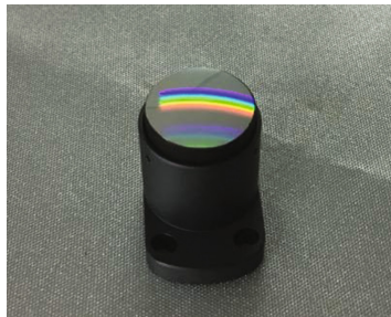
Fig. 5. The fabricated convex blazed grating
