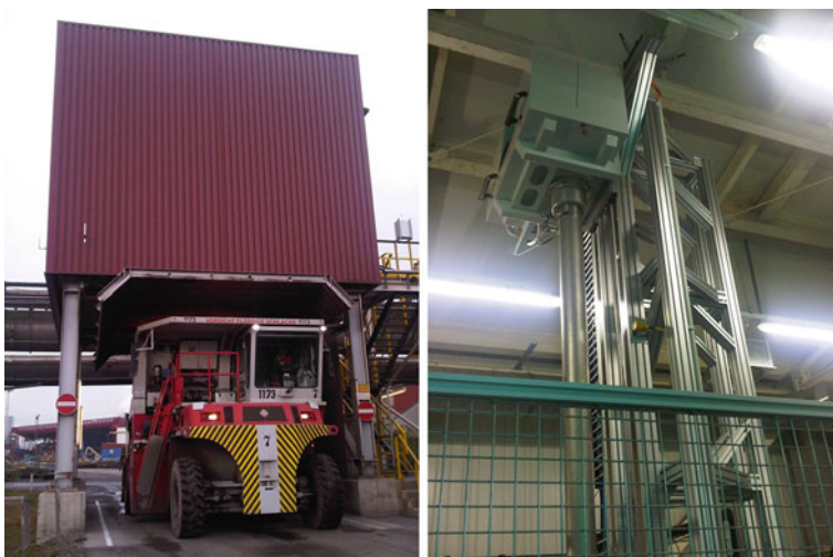
Fig. 13.14 Left Measuring system based on laser material analysis—mounted inside the red cabin —for the inline determination of the basicity of liquid slag originating from a steel plant and transported in a bucket with a truck stopping underneath the measuring system. Right Inside view of the cabin with the laser measuring system mounted at a scaffolding and coupled to a measuring lance ( cylindrical tube ) enclosing the laser beam being directed downwards to the slag surface in the bucket. Fotos by courtesy of voestalpine
