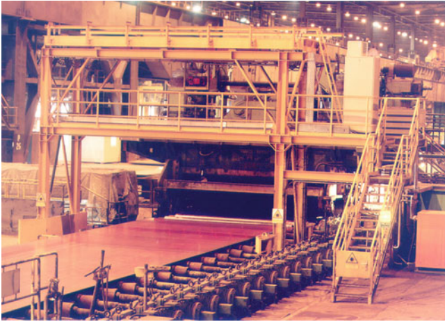
Fig. 10.25 Flatness measurement system based on laser triangulation in a rolling mill
