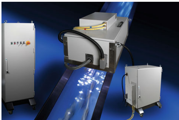
Fig. 13.12 System for the identification of scrap pieces transported on belt conveyors. Left electric control cabinet, middle laser module mounted above the belt conveyor with scrap pieces and laser-induced plasmas (time exposure comprising a set of measurements), right spectrometer module linked with the laser module via fiber optics
