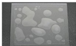
Fig. 22.1 Touch panel devices and bubbling issue of plastic panels
