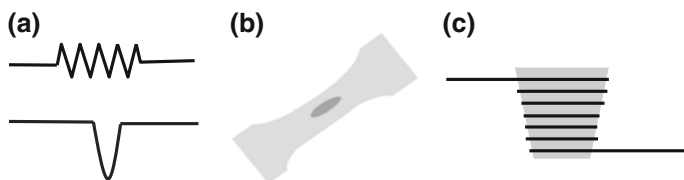
Fig. 2.3 Scheme of different heating elements to evaporate by resistance heating: a tungsten filaments, b metal boat and c ceramic crucible
