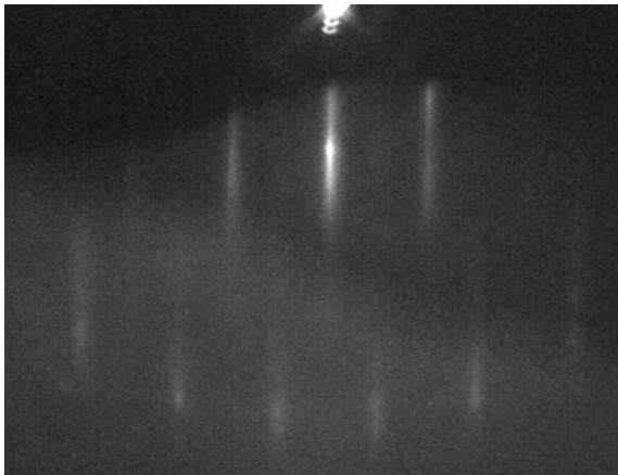
Fig. 2.10 The 1 \times 1 RHEED (reflection high-energy electron diffraction) pattern measured in situ on the 5 QL (\text{Bi}_{0.12}\text{Sb}_{0.88})_2\text{Te}_3 film grown by MBE. The sharpness of the pattern indicates the high quality of the sample
