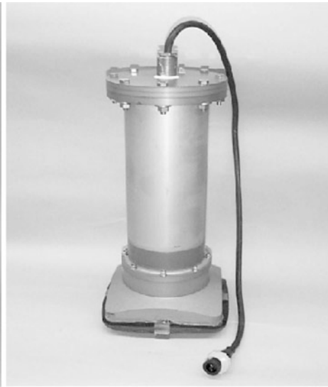
Fig. 1.16 A high power magnetostrictive/piezoelectric hybrid transducer with square piston, piezoelectric ceramic drive, centermass, magnetostrictive drive, and tail mass along with water-tight housing and electrical connector [34]
