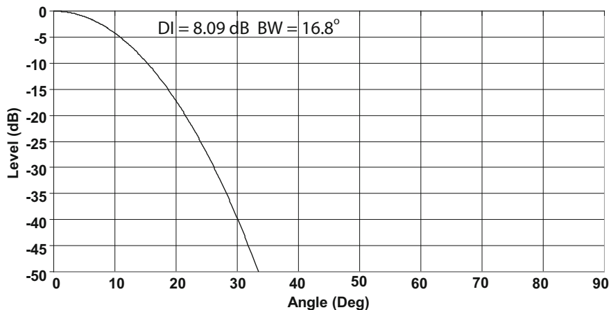
Fig. 8.6 12 element \lambda/2 spaced array with binomial shading. Coefficients: 1, 0.714, 0.357, 0.119, 0.024, 0.002
