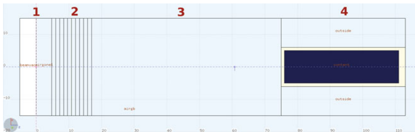
Figure 3.1: FLUKA model of the RPTC beamline, as described in Englbrecht [2014]. The proton beam, coming from the left, exits the vacuum (white) through the vacuum window (1), crosses the multi strip ionization chamber (MSIC) and transmission ionization chamber (TIC) (2) and propagates through the air-gap (3) between the nozzle and the patient table, where arbitrary phantoms can be placed (4).
