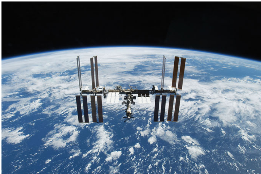
Fig. 2.1 The International Space Station is a joint venture between several countries. The first part of it was put in orbit in 1998 and several modules have since been added. It now measures 108 m across and 88 m long, and has almost half a hectare of solar panels to power it. It orbits Earth at an altitude of 400 km (Credit: NASA/ISS).
