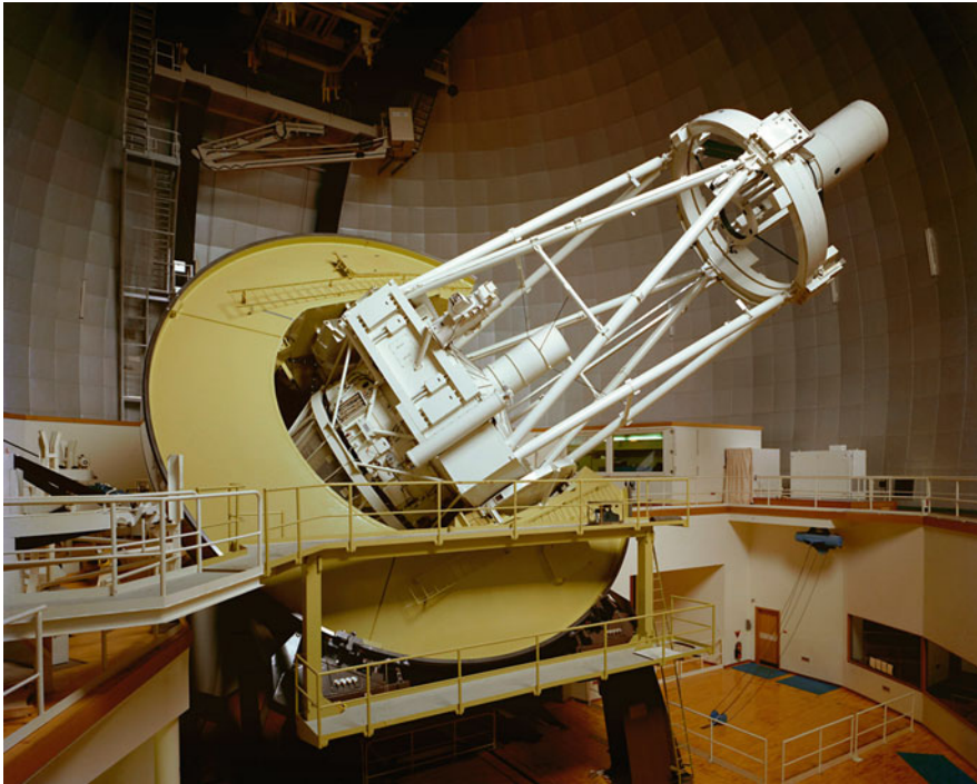
Fig. 1.2 Astronomers use optical telescopes to explore the universe. Pictured is the 3.9 m diameter Australian telescope on Siding Springs Mountain, Australia (Credit: Australian Astronomical Observatory/David Malin).
