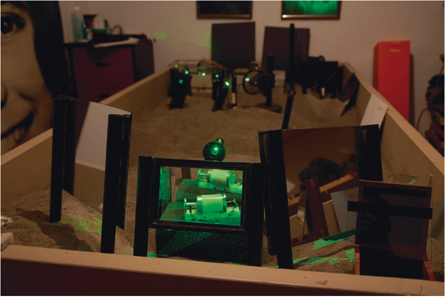
Setup for making a hologram of the first laser; holography was “invented” by physicist Dennis Gabor in the late 1940s (and awarded a Nobel Physics prize in 1971), but the process became feasible only after invention of the laser in 1960. Courtesy of Gary Cullen
