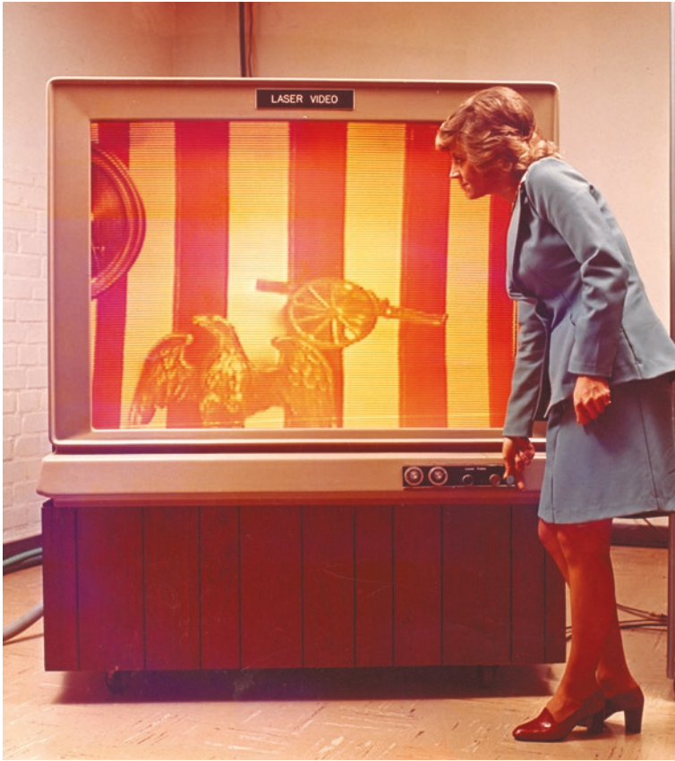
Large-screen video display unit developed in Ted's company Laser Video Inc., operating and patented in 1976, screen 45 inch \times 60 inch (about 1.2 meter \times 1.5 meter). ©Maiman Archive
