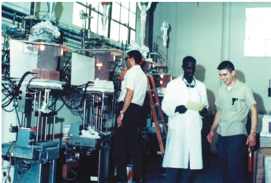
Korad Lasers staff workers tending to Verneuil furnaces for growing ruby crystals, 1960s. ©Maiman Archive
