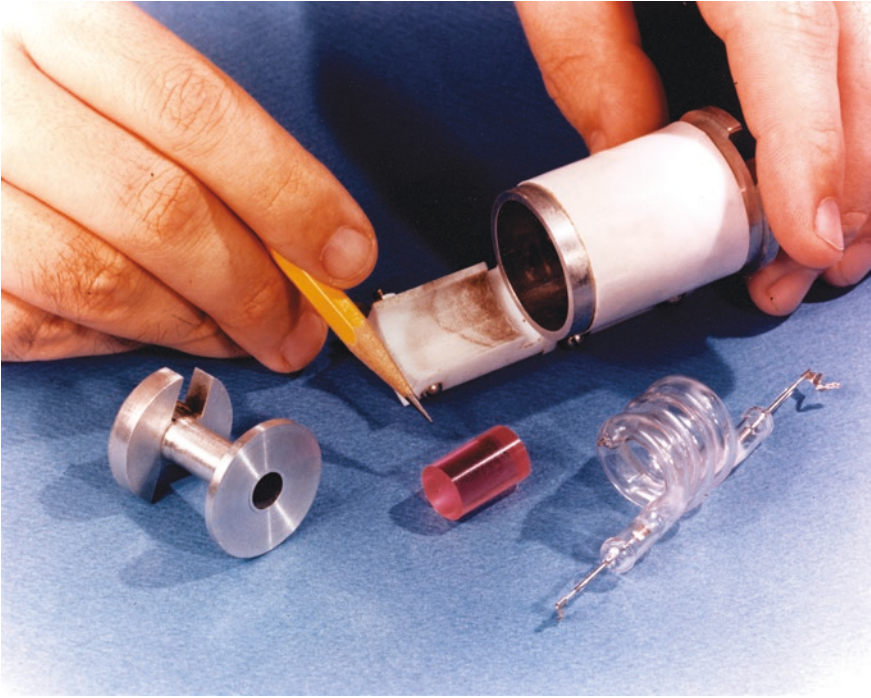
Ted holding the original laser with parts disassembled. ©Maiman Archive
