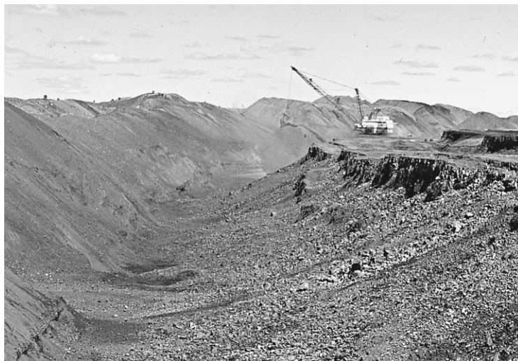
FIGURE 8.1. An example of an open-cut coal mining operation where massive drag-lines are used to strip away soil and over-burden and expose the coal layer.
