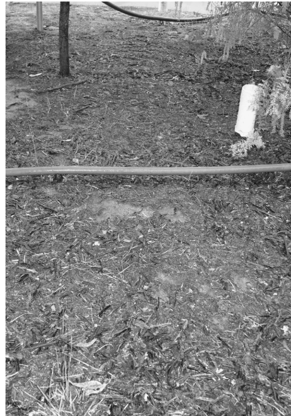
FIGURE 10.9. During rainfall simulation experiments, litter and woody debris within tree belts provided high surface resistance to flows of water and also filtered out soil particulates.
