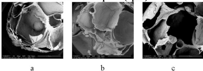
Fig. 11.4 Effect of process conditions and material characteristics on the microstructure of extrudates: (a) ( C=7.5\% , T=160\text{ }^{\circ}\text{C} , N=200\text{ rpm} ) (a) X=14\% , (b) X=17\% , (c) X=20\% ; (b) ( X=17\% , T=160\text{ }^{\circ}\text{C} , N=200\text{ rpm} ) (a) C=5\% , (b) C=7.5\% , (c) C=10\% ; (c) ( X=17\% , C=7.5\% , N=200\text{ rpm} ) (a) T=140\text{ }^{\circ}\text{C} , (b) T=160\text{ }^{\circ}\text{C} , (c) T=180\text{ }^{\circ}\text{C} ; (d) ( X=17\% , C=7.5\% , T=160\text{ }^{\circ}\text{C} ) (a) N=150\text{ rpm} , (b) N=200\text{ rpm} , (c) N=250\text{ rpm}
