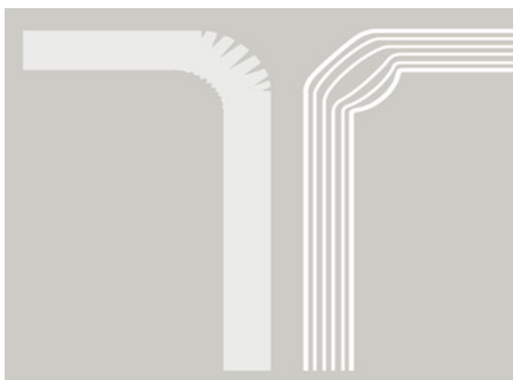
Fig. 6.5 Multi-ply structures offer higher folding performance as a result of plies layering
