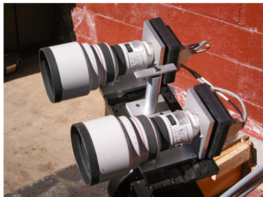
FIG. 5.15 The XO-instrument contains two 20 cm telephoto lenses, each with its CCD camera (NASA/ESA /J. Stys/STSci)
