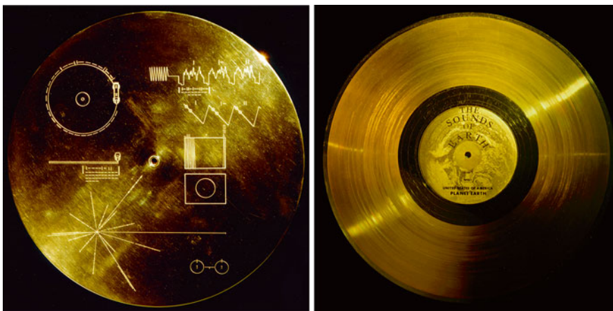
FIG. 8.5 The golden record carried by the Voyager spacecrafts. To the left is seen the cover with basic instructions and information, to the right the actual record (NASA)
