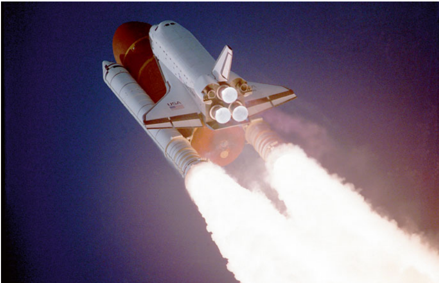
FIG. 12.2 Take-off for the space shuttle Atlantis. The two booster rockets contains solid fuel, while the red tank contains liquid fuel to the engines of the actual shuttle (NASA)
