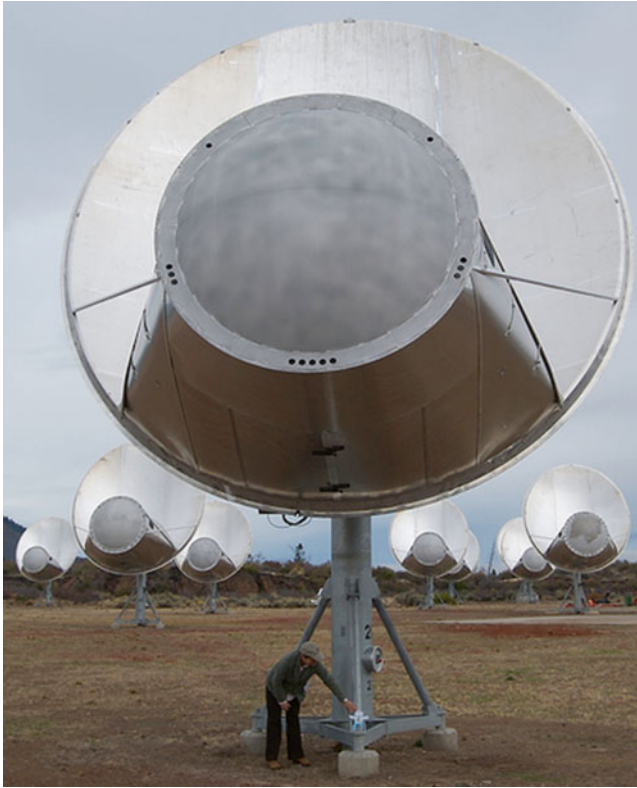
FIG. 11.10 Close-up view of one of the antennae of the Allen telescope, which consists of a number of interconnected disks, each with a size of 6 m (Colby Gutierrez-Kraybill)
