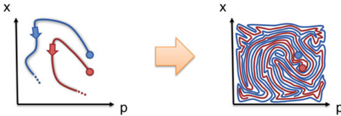
Fig. 3.2 A sketch of classical ergodicity. Thermal equilibrium is independent of the initial state of a non-equilibrium evolution. After a sufficiently long time, both initial trajectories come arbitrarily close to any point in the position-momentum ( x - p ) phase space. This leads to the law of equal a priori probabilities for all microscopic states within a certain energy window. In the process, all memory of the initial state is dynamically erased
