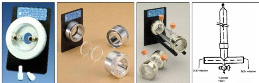
**Fig. 10.3** Cells for infrared analyses: sealed, collapsible, for gas and high vacuum
