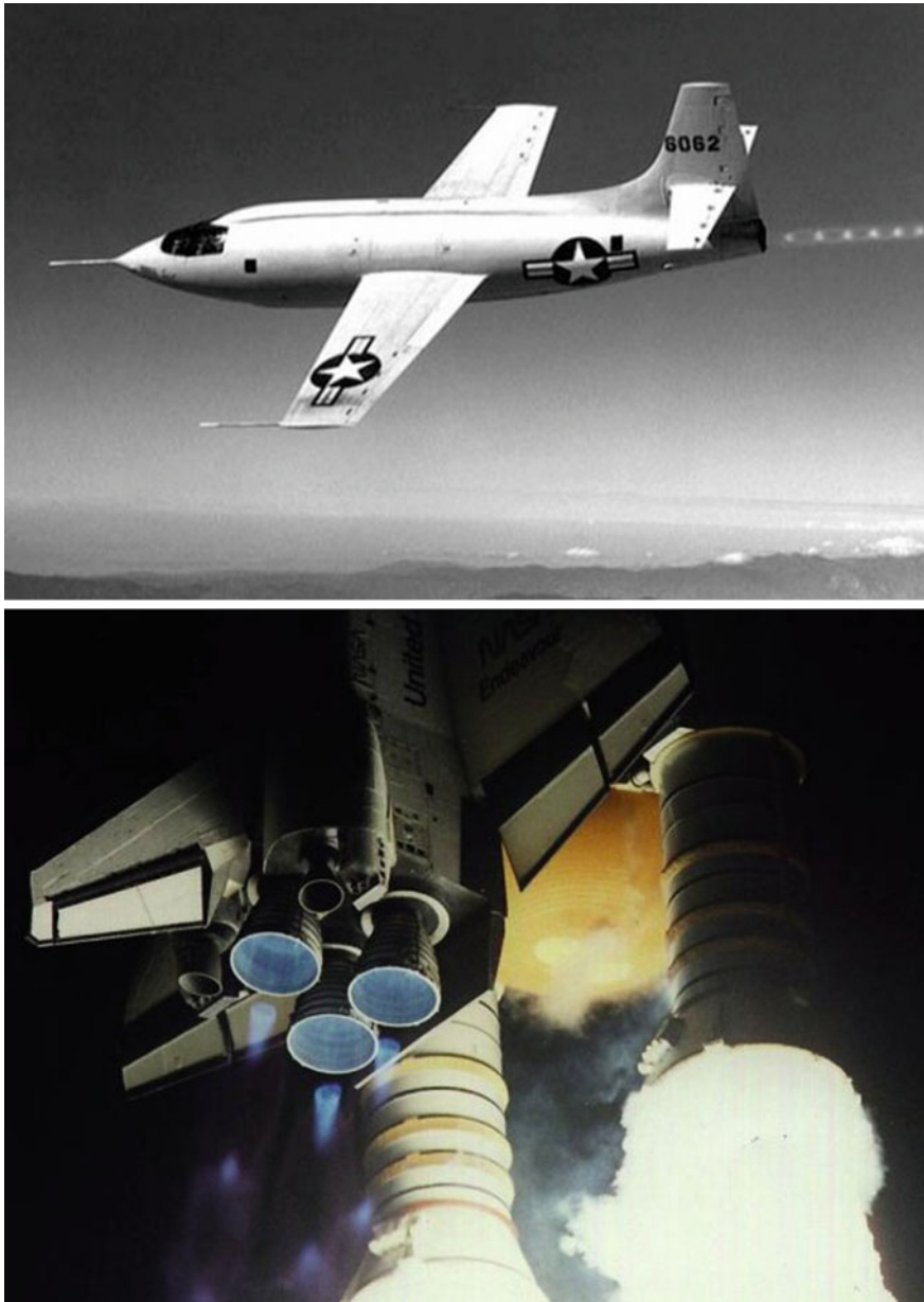
Fig. 10.2 Mach disks in the exhaust jet of the Bell X-1 rocket plane ( top ), and behind the three main engines of the Space Shuttle ( below ). Behind the Bell X-1 a series of bright 'blobs' are visible. These show the location of the series of Mach disks. Behind the Shuttle engines, only the first Mach disk is clearly visible, the following Mach disks in the series are less distinct
