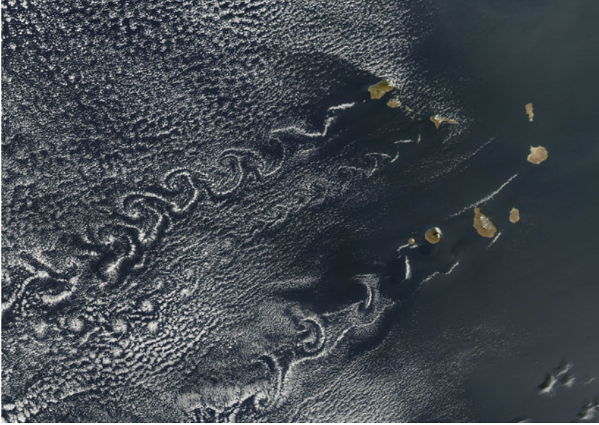
Fig. 5.8 The shedding of vortices in the wind wake of the Cape Verde Islands off the coast of North Africa. The vortices are visible because of the fleecy clouds that follow the flow
