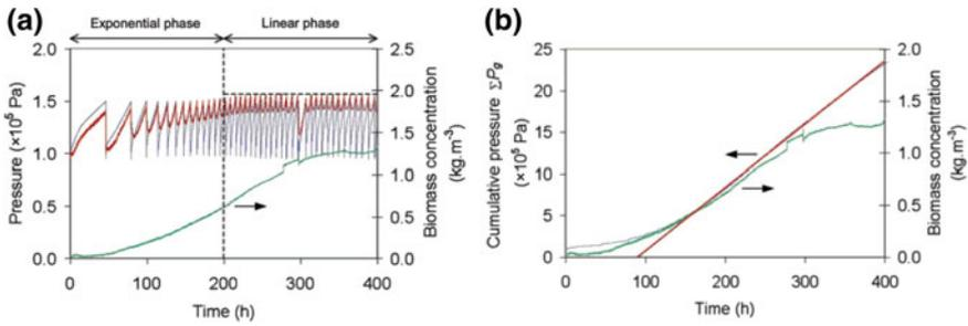
**Fig. 14** **a** Biomass concentration and overall pressure in the gas phase during cultivation of *Arthrospira platensis* in this novel membrane-aerated photobioreactor. **b** Cumulative pressure representing  $\text{O}_2$  production during cultivation [103]
