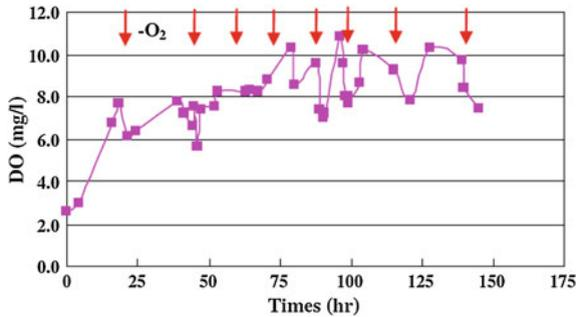
**Fig. 16** Dissolved O<sub>2</sub> profile during cultivation. Arrows indicate switching on the vacuum pump to start the membrane module for O<sub>2</sub> removal [104]
