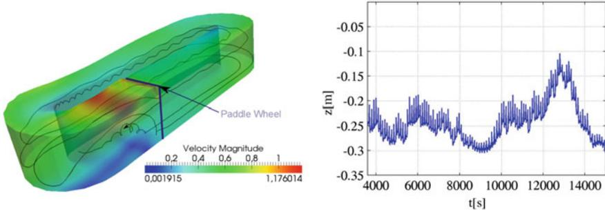
**Fig. 6** 3D Representation of the velocity field in a raceway pond along with a particular cell trajectory (*left plot*), and variation of the depth of a single cell over time (*right plot*). Reproduced from [52]
