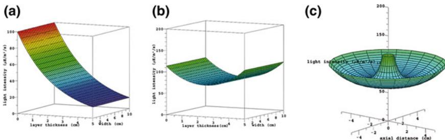
**Fig. 8** Typical light intensity distribution in different reactor types for a light intensity of  $100 \mu\text{E}/(\text{m}^2 \cdot \text{s})$  and same absorption coefficients  $\epsilon$  and layer thickness  $D$ . **a** Single-sided illumination of a plate-type reactor; **b** double-sided illumination of a plate-type reactor; **c** cylindrical reactor with outside illumination [72]
