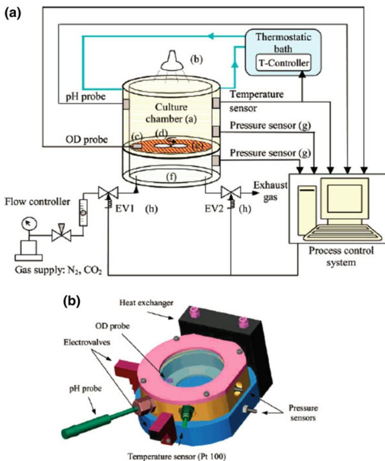
**Fig. 13** **a** Scheme of the reactor and its periphery. **b** Online measurements with the help of sensors for pH, OD, and pressure [103]
