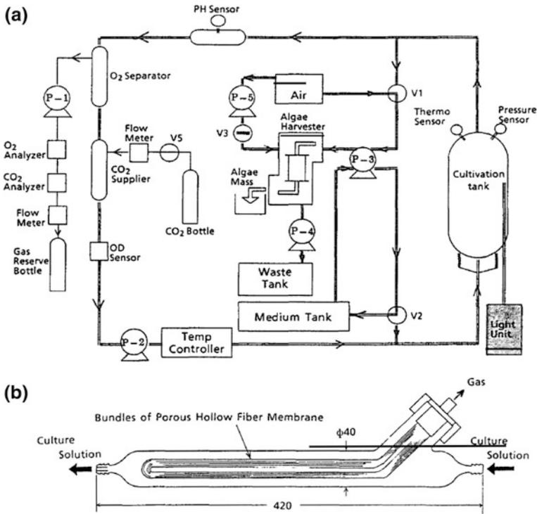
**Fig. 20** a Scheme of photobioreactor system for CELSSs proposed by Oguchi et al. [107]. b Gas separator used in this approach with an effective area of  $0.3 \text{ m}^2$
