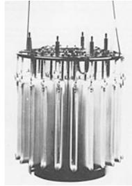
**Fig. 11** Diessel reactor with porous Accurel PP hollow-fiber membranes coiled and fixed on carriers [99]. In the production reactors with 20 and 150 l membrane coils were driven eccentrically (for 1 L scale a pendulous motion was applied) and to have homogeneous mixing of microcarriers a spiral agitator was fixed below the membrane carriers
