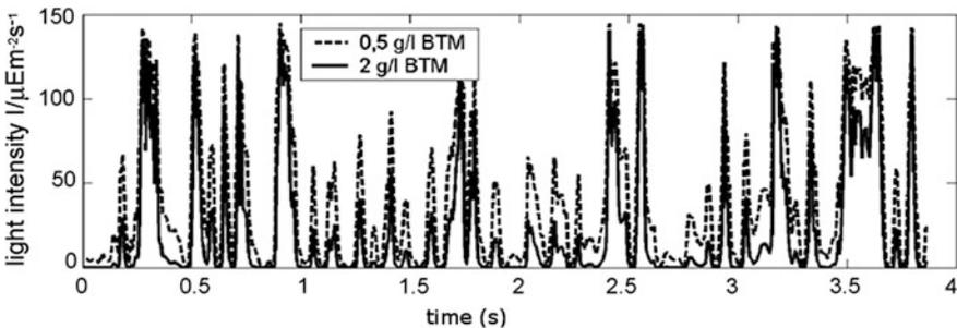
**Fig. 9** Simulated light patterns received by a microalgae cell in a tubular photobioreactor at two different cell concentration levels:  $0.5 \text{ g L}^{-1}$  (dashed) and  $2 \text{ g L}^{-1}$  (solid). Reproduced from [80]
