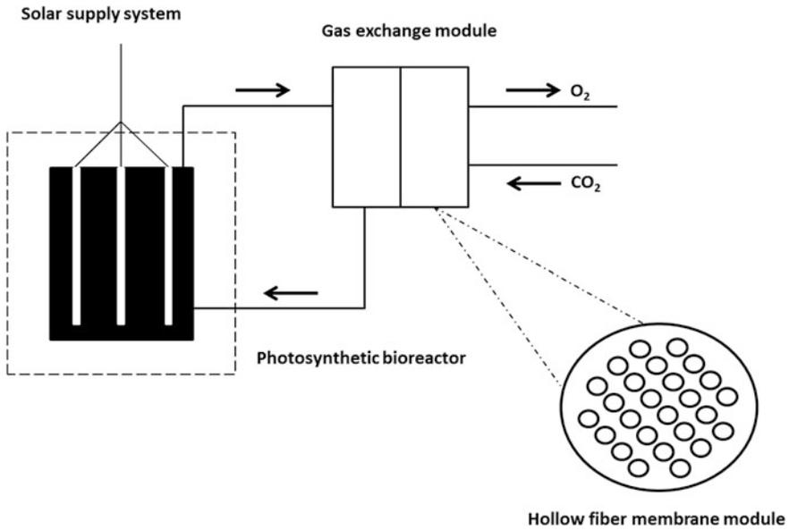
**Fig. 21** Approach for a space photobioreactor by Mori et al. Scheme of proposed system with hollow-fiber membrane module for gas exchange. Modified after [108]
