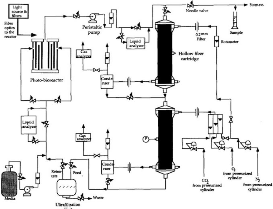
**Fig. 18** Photobioreactor concept for application on CELSSs [15]
