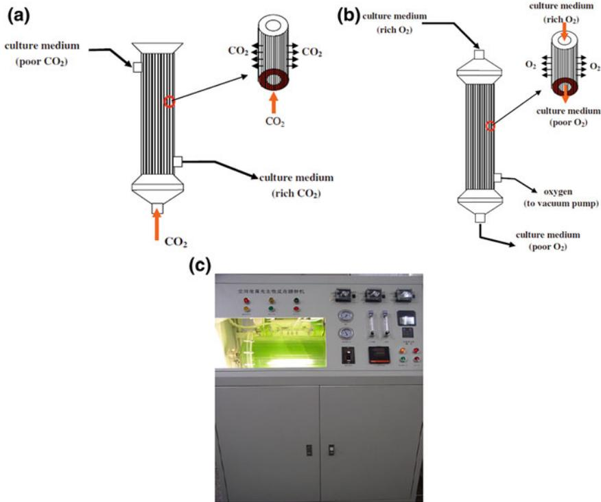
**Fig. 15** **a** Membrane unit for supply of  $\text{CO}_2$ . **b** Unit for removal of  $\text{O}_2$ . **c** Outlook of the developed reactor [104]
