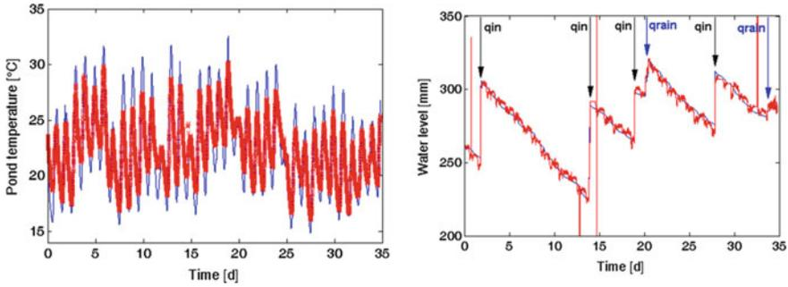
**Fig. 7** Simulation of the temperature evolution in a raceway (blue line) using a model [6] and comparison with experimental measurements (red lines). On the right-hand side, the water level is also represented, with the indication of the water supply ( $q_{in}$ ) and rain ( $q_{rain}$ )
