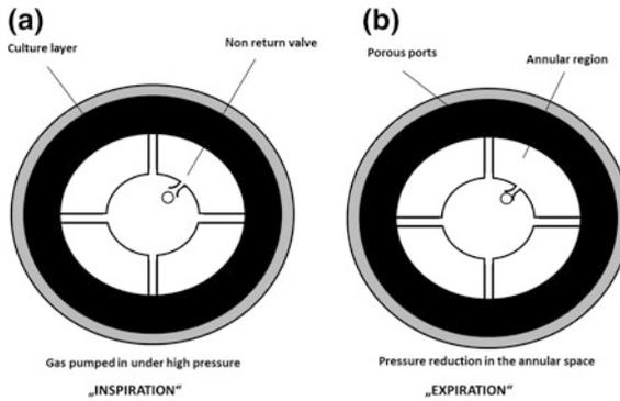
**Fig. 17** Scheme of the pseudo-rotating bioreactor aeration concept for bubble-aeration using artificial gravity for gas-liquid separation. Modified after [106]
