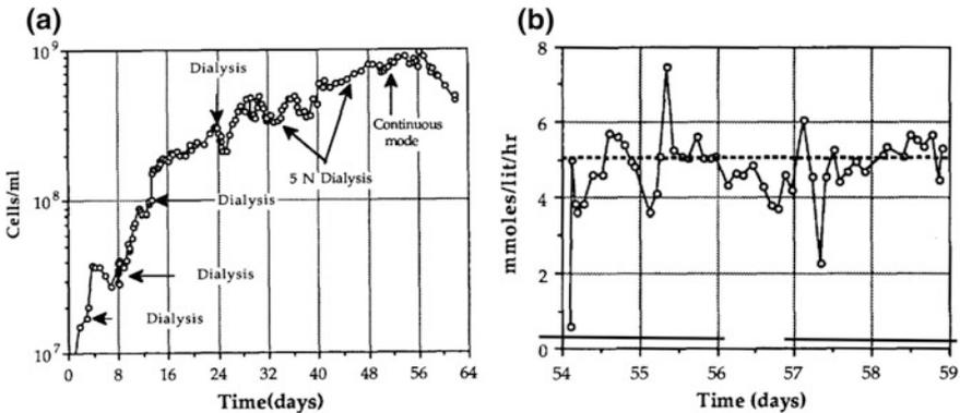
**Fig. 19** Growth curve showing batch and continuous phase of cultivation (a) and volumetric OPR versus time (b) during steady state of continuous mode in photobioreactor designed for CELSS [15]
