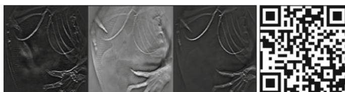
Fig. A.2 Supp. Mov. 2. From left to right Absorption, phase and dark-field contrast tomosynthesis of a formalin-fixed lizard. Note the superior depiction of the scales and the organs in the phase and dark-field channel, respectively. Available: https://www.youtube.com/watch?v=A8A52_KvSQE
