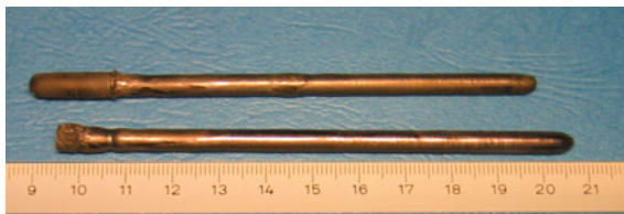
Fig. 4.3 Typical \text{Na}_{0.82}\text{CoO}_2 (upper) and \text{Na}_{0.75}\text{CoO}_2 (lower) single crystal ingots obtained by the optical floating zone technique
