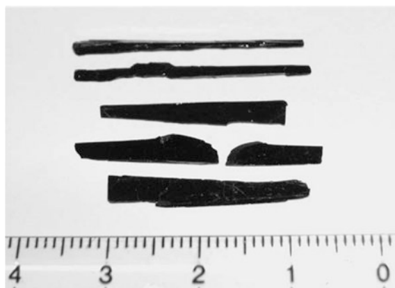
Fig. 3.9 \text{Bi}_{2.13}\text{Sr}_{1.55}\text{La}_{0.43}\text{CuO}_y single crystals cleaved from as-grown ingot [27]
