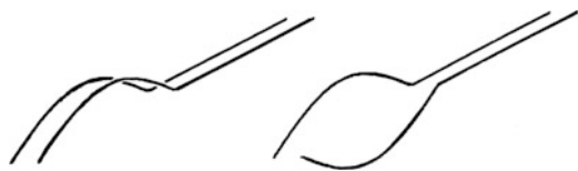
Fig. 4.2 The circulating pulses on the strings when excited in the normal symmetric mode (left) and in the anti-symmetric mode (right)
