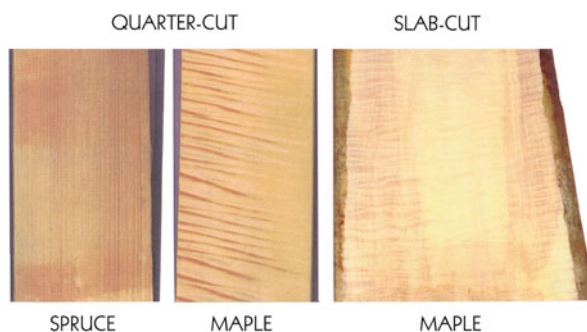
Fig. 5.26 Quarter-cut Dolomite spruce and Balkan maple and slab-cut Balkan maple. The grain is vertical in each case, although the “flaming” in the maple samples is nearly horizontal (photograph by the author)
